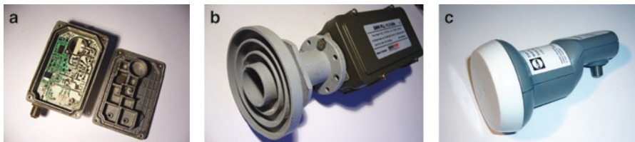
Fig. 10.2. (a) The LNB circuit. This kind of circuit is difficult to make at home. Note that the cover has built-in shielding walls to isolate various parts of the circuit. (b) LNB with a c120 feed horn used on concentric dishes. (c) A European Universal LNB used on offset dishes.
