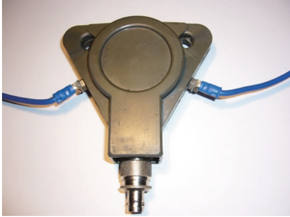
Fig. 11.1. Dipole antenna. This one is based on a commercially made balun. There is an adapter fitted to the base to provide a BNC output. The wire used was a 2.5 mm 2 electrical mains cable. Additional elements can be fitted to increase the bandwidth so long as they are not mutually resonant. For an antenna to work between 18 and 24 MHz use three pairs of wires a total length of 7.94, 6.81, and 5.96 m wide. See Chap. 5 for more information.
