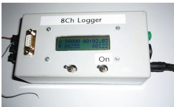
Fig. 10.7. Data logger, this one is based on a kit supplied by Magenta Electronics. There is more on data logging in a later chapter.
