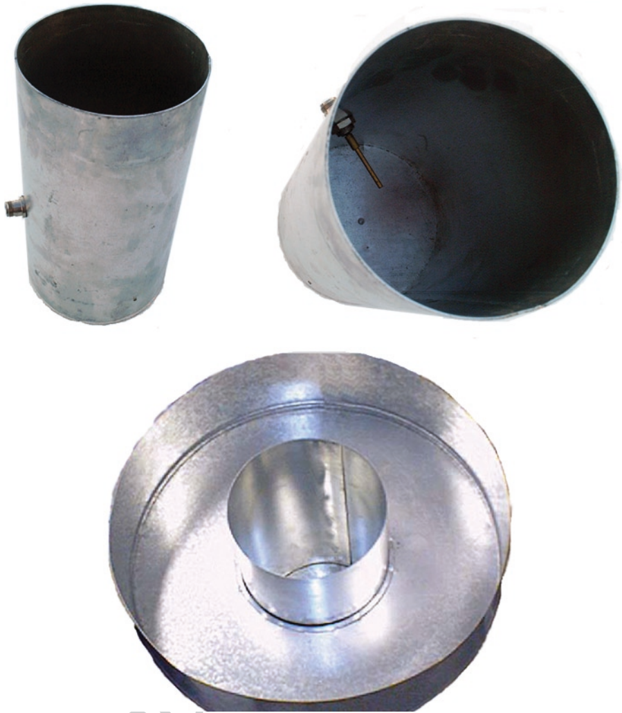
Fig. 5.10. Can-type feed horn for 21 cm hydrogen line.
