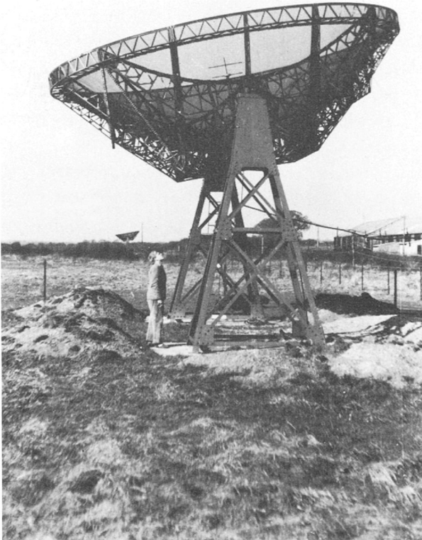
Figure 4. The 7.5 m Würzburg paraboloids in 1950. With this interferometer Graham Smith (pictured) provided the accurate positions which led in 1951 to the identifications of Cas A and Cyg A by W. Baade and R. Minkowski (photo by B. Elsmore).
