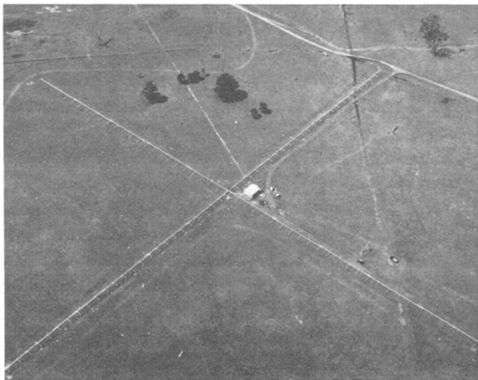
Fig.7 The 85 Mc/s Mills Cross at Fleurs Field Station with arms 1500 ft long.
