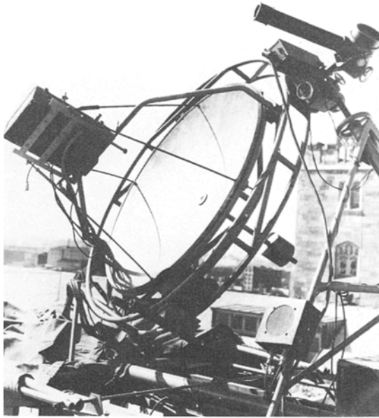
Fig.5 Piddington and Minnett's 1.25 cm tracking antenna for measurement of the surface temperature of the Moon, 1949.
