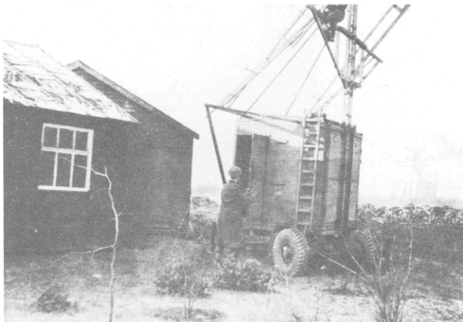
Figure 1 : The first day at Jodrell Bank - mid-December 1945. The receiver cabin of an Army 4.2 metre radar. The Yagi aeriels are on the roof. The wooden huts contained the fertilisers and tools of the two gardeners working in the botanical grounds.
