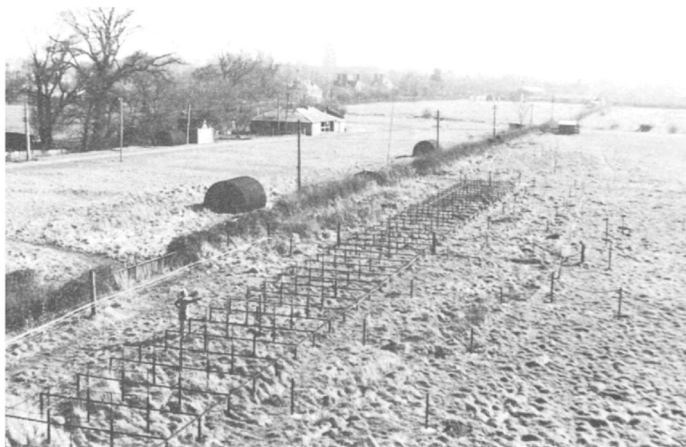
Figure 1. One of the elements of the "Long Michelson" interferometer, a broadside array operated at 3.7 m wavelength on the Old Rifle Range in Cambridge (ca. 1950). This instrument produced the LC survey of radio stars. Martin Ryle's house can be seen just to the right of the tower of the University Library in the distance.
