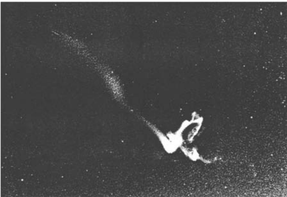
Figure 10.3 Photograph of a sodium vapor trail released from a sounding rocket showing the transition from a turbulent to a diffusive region in the atmosphere. 9
