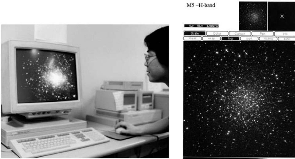
Figure 10.2. A computer screen and a display package (SAOimage) to allow digital images to be displayed and enhanced.
