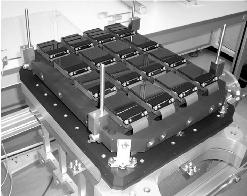
Figure 11.18. An array of 162\text{ K} \times 2\text{ K} HgCdTe (Raytheon) detectors for the VISTA telescope on Cerro Paranal (Chile). Credit: STFC.
