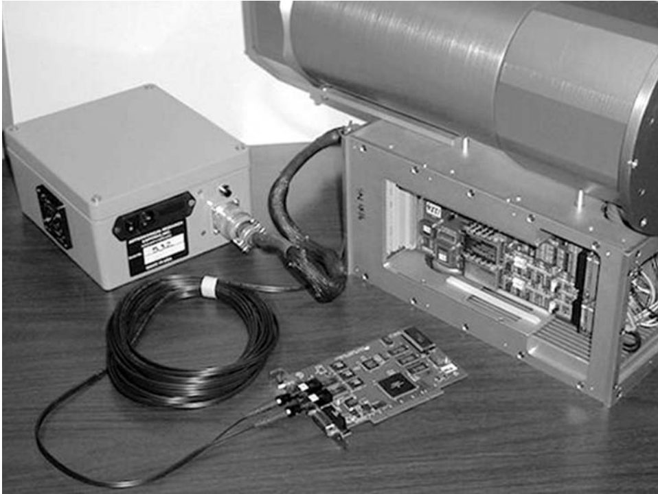
Figure 8.5. A typical camera “head” electronics box and CCD controller. This one shows the system developed by Astronomical Research Cameras. Credit: Bob Leach.
