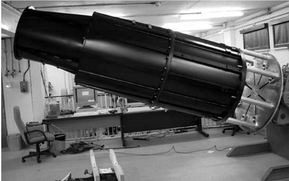
Figure 11.15. The Wide-Field Camera (WFCAM) for the 3.8 m UKIRT undergoing tests in a lab prior to delivery. This large instrument has four 2\text{ K} \times 2\text{ K} HgCdTe arrays. Credit: ROE/ATC.
