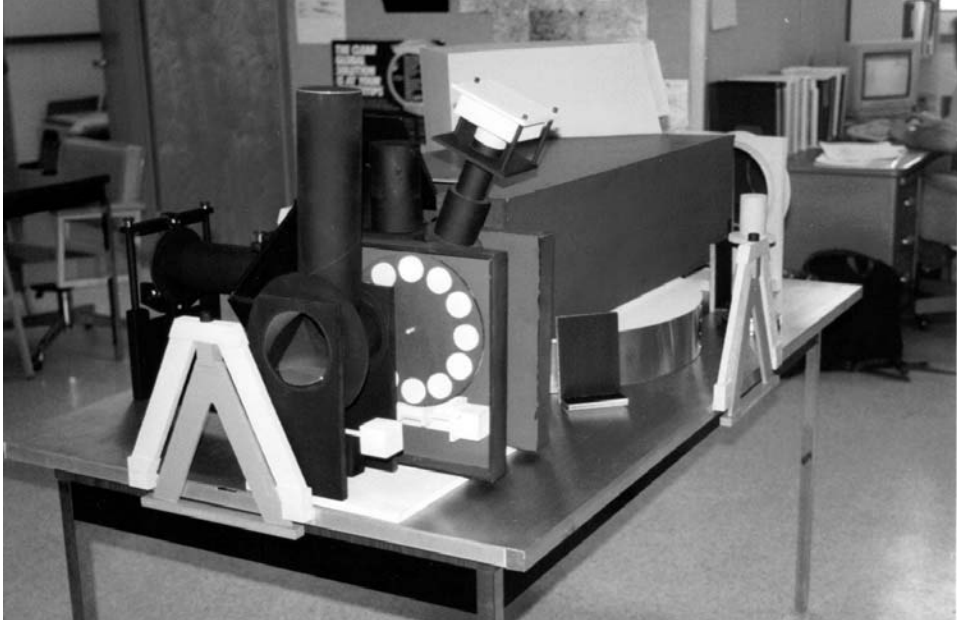
Figure 6.7. A “space” model of an infrared spectrograph constructed at the IR Lab at UCLA.
