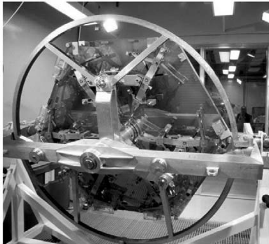
Figure 3.11. Arrangement of the 36 hexagonal segmented mirrors in the Keck primary is shown together with a close-up view of one of the segments. This single segment is mounted on its handling frame prior to aluminizing. The glass is Zerodur and the segment is 0.9m along each edge or 1.8m from opposite tips. Credit: Jerry Nelson and WMKO.
