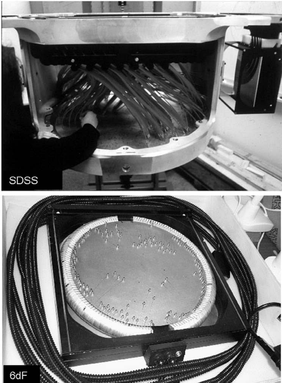
Figure 4.16. Two fiber systems: at the top is the “plug-plate” for 600 fibers in the Sloan Digital Sky Survey. Credit: SDSS. Bottom: a fiber-optical system called 6dF that robotically positions small prisms and fibers to a plate that is inserted into the wide-field U.K. Schmidt Telescope. Credit: AAO.
