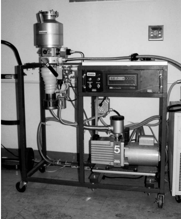
Figure 6.12. A pumping station with a diffusion pump (vertical stack) and a roughing (rotary) pump in the lower right.
