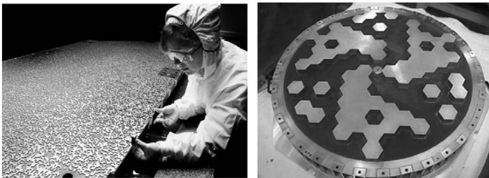
Figure 12.3. (Left) The random coded mask telescope for the SWIFT gamma-ray satellite; and (right) the cyclic coded mask for the INTEGRAL gamma-ray satellite. Credit: SWIFT and INTEGRAL Teams.
