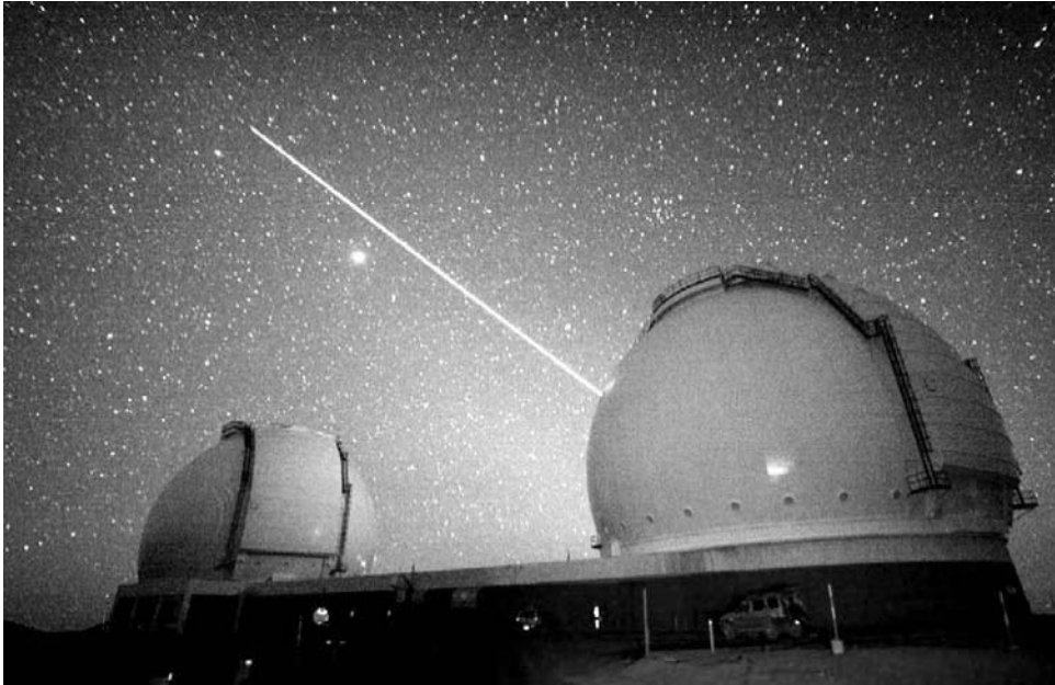
Figure 2.13. A long-exposure picture of the sodium laser beacon projecting from the Keck II telescope. Credit: WMKO. See also Plate 9.
