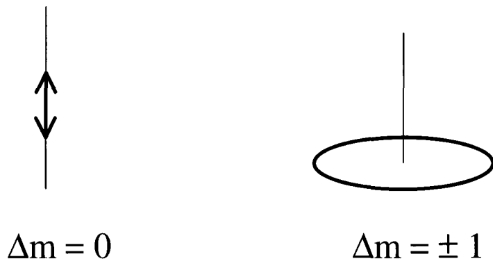
FIGURE 9. Polarization properties of different \Delta m transitions.
