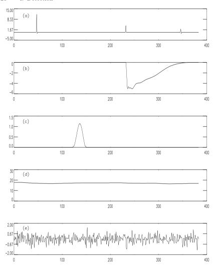
**Fig. 4.8.** Decomposition of the signal into its main components: (a) short glitch, (b) glitch negative tail, (c) source, (d) baseline, (e) noise. The simple sum of the five components is exactly equal to the original data (see previous figure). The calibrated background-free data are obtained by addition of signals (c) and (e).
