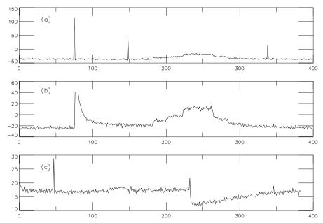
**Fig. 4.6.** Examples of glitches. (a) This signal contains three glitches of the first type. (b) A glitch with a long tail appears (named fader) around the position 80. The glitch has been truncated, and its real amplitude is 2700 ADUs. (c) A glitch with a negative tail (named dipper) appears around position 240.
