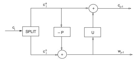
Fig. 5.11. The lifting scheme – forward direction.
