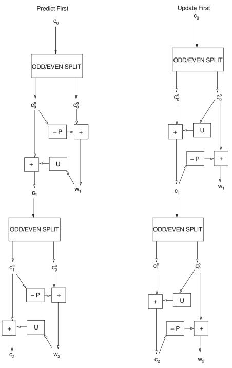
${f Fig.~5.12.}$  The lifting scheme with two iterations: left, predict-first approach, and right, update-first approach.
