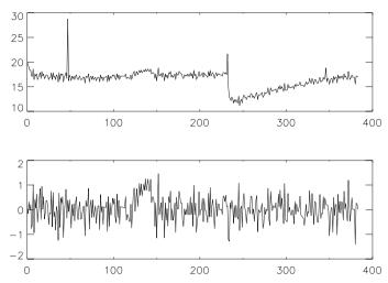
**Fig. 4.7.** Top: original data, and bottom: calibrated data (background free). The flux in ADUs (analog to digital units) is plotted against time given by the number of exposures. Note the gain variation of about 5 ADUs which appears after the second glitch.
