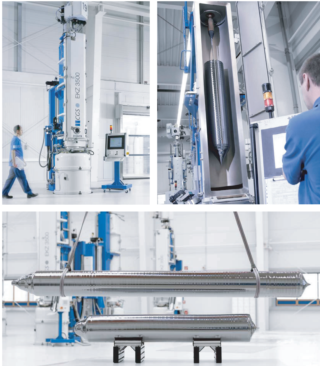
FIGURE 33 Silicon crystal growing machine, and two resulting crystals, with a length of c. 2 m (© www.PVATePla.com )
