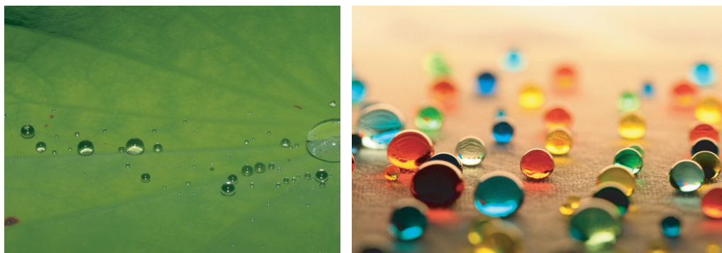
FIGURE 43 The beauty of materials science: the surface of a lotus leaf leads to almost spherical water droplets; plasma-deposited PTFE, or teflon, on cotton leads to the same effect for the coloured water droplets on it (© tapperboy, Diener Electronics)
