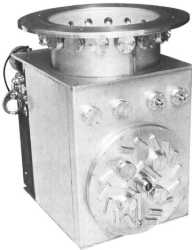
FIG. 8. Pumping module with demountable array installed. Overall height of the module is 84 cm and the baseplate diameter is 66 cm.
