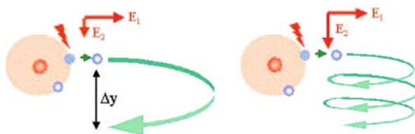
Fig. 4 Illustration of the trajectory of the electron in elliptically polarized light. The left panel shows how a small amount of elliptical polarization causes the just-detached electron to move laterally, so that it is less likely to recollide with the parent ion. The right panel illustrates circularly polarized light, whereby the electron trajectory never returns to the parent ion. By means of controlling the ellipticity of the laser light, one can control the electron trajectory or even turn off the recollision process. This technique is important in clarifying the shape of the electron wave packet and its influence upon recollision
