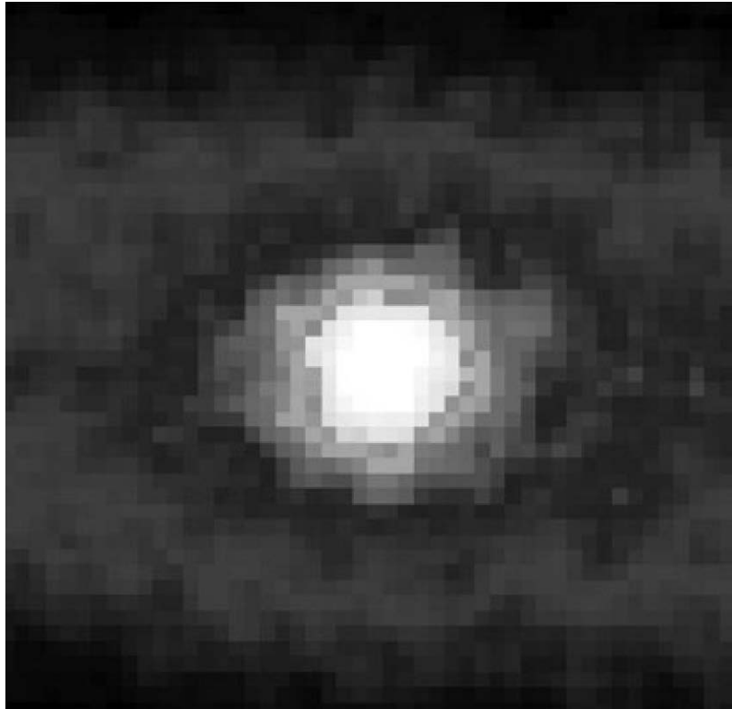
Figure 9 Neutrino-graphy of the Sun. The Sun as 'seen' when its neutrinos are detected.
