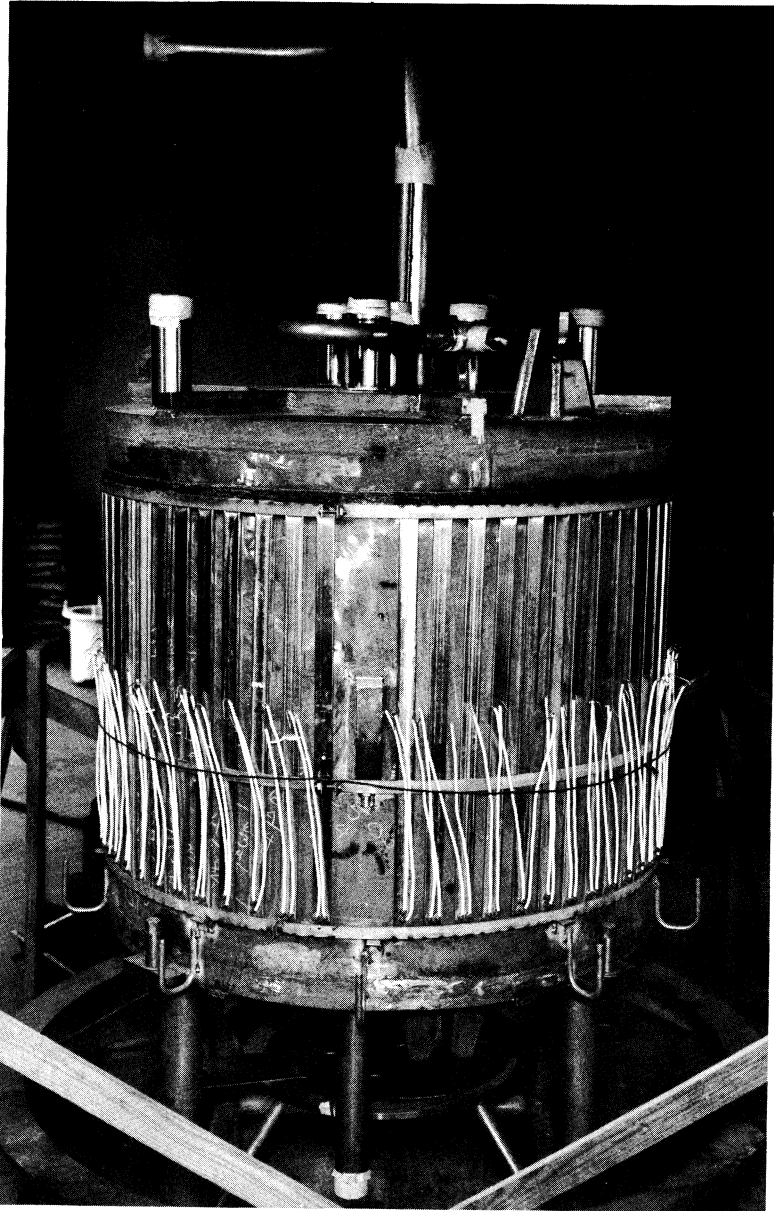
FIG. 16-3. View of the ARE Vessel before addition of the thermal shield. The external strip heaters with their electrical leads are shown in place.
