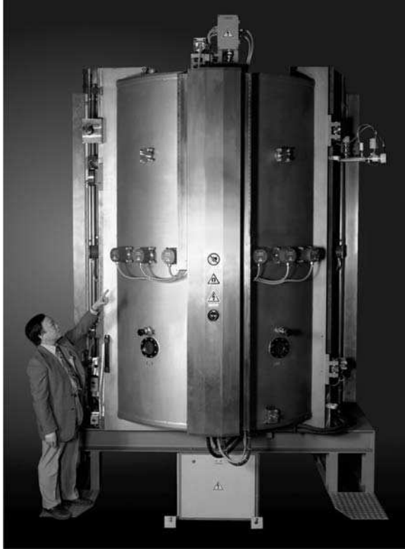
Fig. 5.39. Very large batch coater capable of coating large batches or very large individual parts. (Photo courtesy of Hauzer Techno Coatings)
