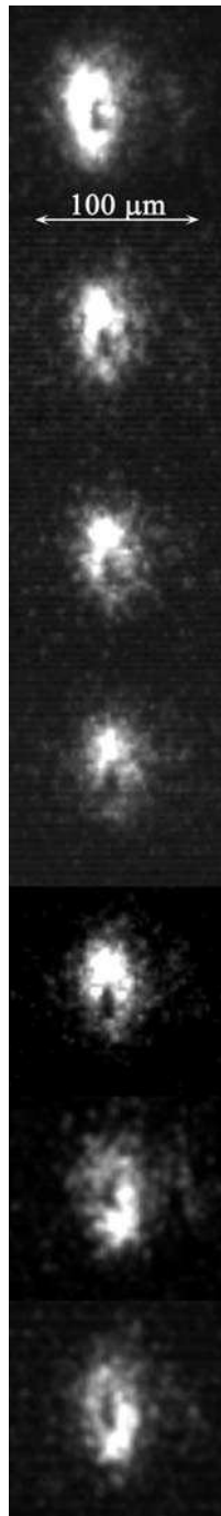
Fig. 3.30. High-resolution imaging of spot fragments igniting preferably on the asperities of a large cathode. Copper cathode, arc current 30 A, frame exposure time 10 ns, first frame taken 300.00 \mu s after arc triggering. (Courtesy of B. Jüttner, [140])
