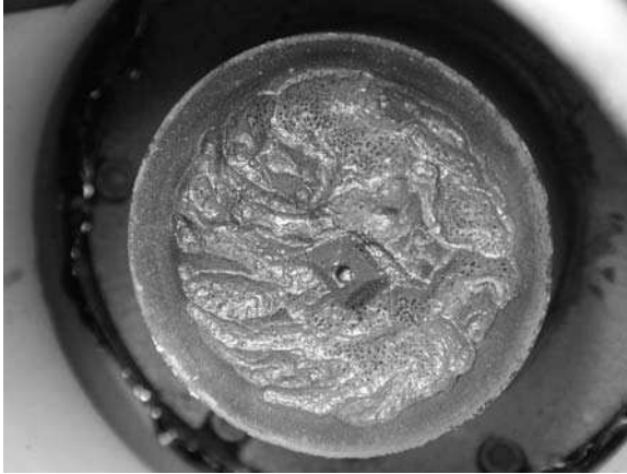
Fig. 5.19. Boron cathode produced by the microwave sintering process [25], shown here after arc operation. (Courtesy of C.C. Klepper, HY-Tech Corporation)
