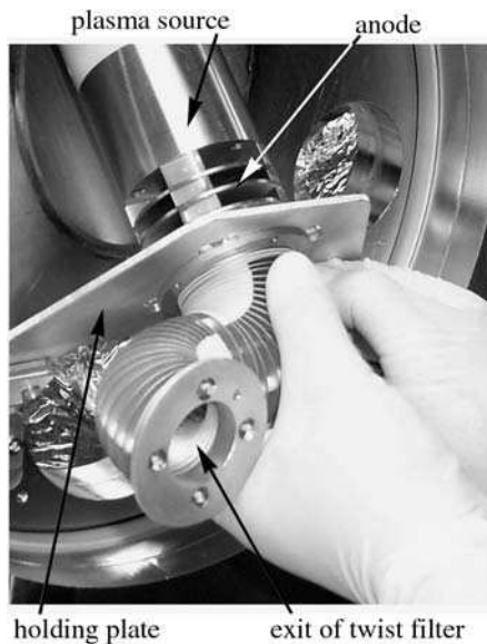
Fig. 7.28 Compact twist filter for the pulsed deposition of ta-C films; the system offers a source with advancing graphite cathode (only the source body is visible here) operating with pulses of about 1 kA, 1 ms, up to 5 pulses per second; this version of the twist filter has flat-shaped turns to promote the reflection of macroparticles from the filter volume. The hands mounting the source give an impression of the extreme compactness of the system, (Photo 2001, Berkeley Lab)
