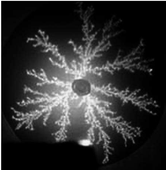
Fig. 5.23. Arc spots moving away from the central trigger of a high-current arc; also here one sees the superposition of random and steered spot motion. (Photo courtesy of Thomas Schülke)
