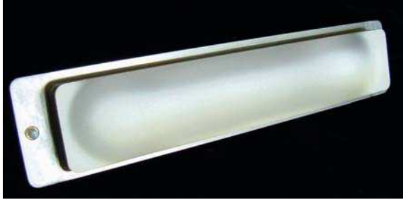
Fig. 5.37. Long (1 m) titanium cathode showing uniform erosion along its length, indicative for uniform plasma production averaged over time. (Photo courtesy of Vergason Technologies, Inc.)
