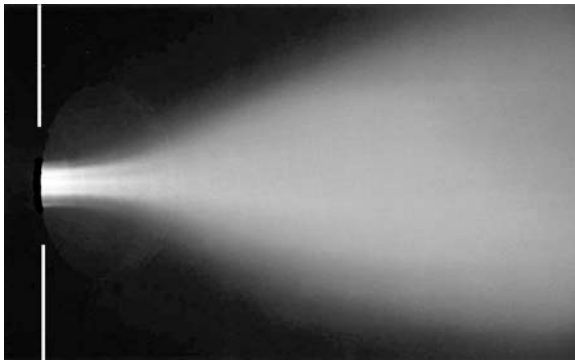
Fig. 6.23. Plasma pluming from the flange-mounted source ( left ) into the chamber (substrates to the right ); the plume is guided by a magnetic field and therefore the coating is improved due to relatively reduced incorporation of macroparticles
