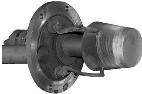
Fig. 2.24. Bulat-3 cathodic arc source, the “workhorse” of large-scale industrial coatings in the Soviet Union; one can see the two trigger electrodes and the conical shape of the cathode, which facilitated spot steering in the axial magnetic field provided by an external coil. (Photo by the author)
