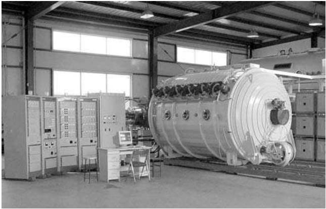
Fig. 5.33. Very large batch coater using a “gang” of point-like arc sources. (Photo courtesy of Dmitry Karpov)
