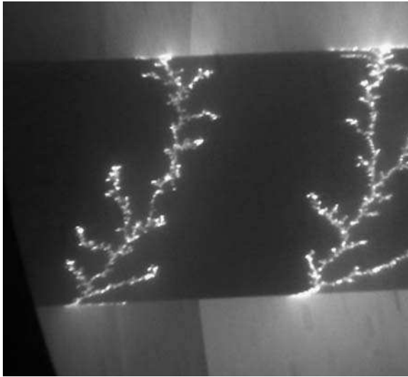
Fig. 5.17. Open-shutter photograph of cathode spots eroding an aluminum rod (diameter 2.5 cm) cathode in vacuum with an axial magnetic field present; the apparent spot motion toward one end of the rod is determined by the electrical contact made to that end of the cathode; one can see the superposition of random branching and steered motion (Berkeley Lab, 2002)
