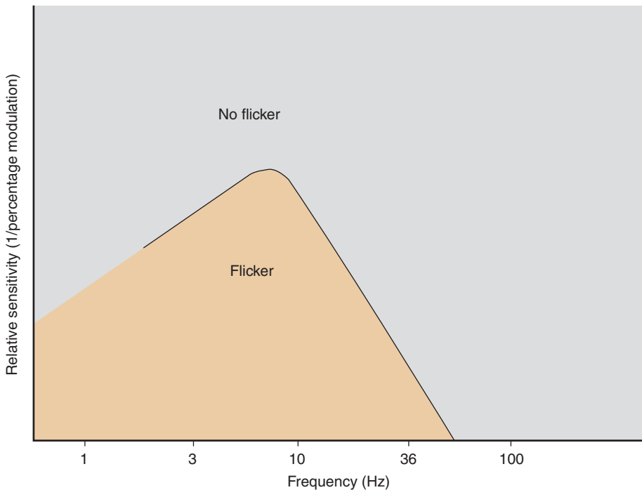
Figure 8–4. Typical temporal modulation transfer function. The graph is plotted on log coordinates.
