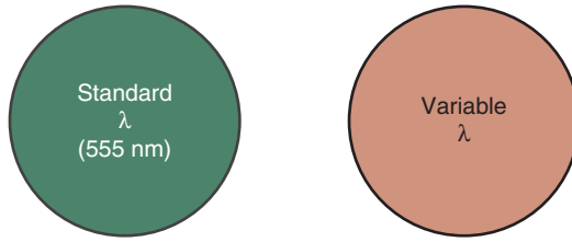
Figure 4-9. Stimulus arrangement for a direct brightness matching experiment. The observer's task is to adjust the radiance of the sample (variable) wavelength such that it matches the brightness of the standard wavelength.
