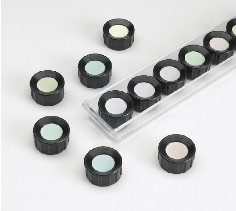
Figure 6-15. Several of the chips used in the Lanthony desaturated D-15 color vision test. (Figure courtesy of Richmond Products, Albuquerque, NM.)
