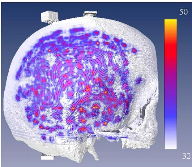
Figure 5: Temperature distribution on the surface skull after 5s sonication.
