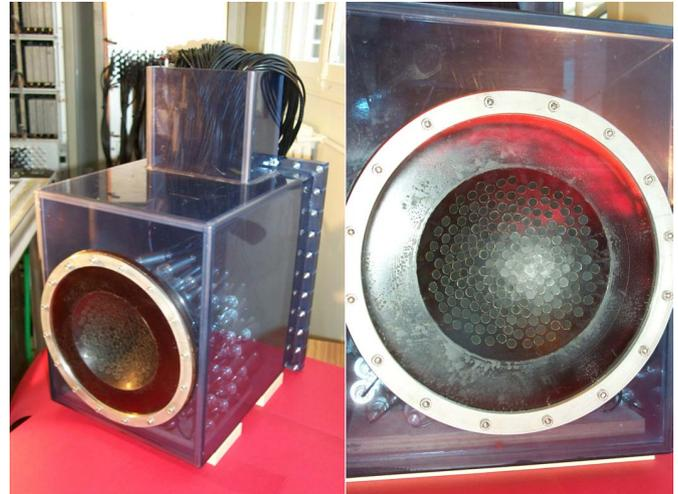
Figure 2. 200-Element high power ultrasonic array.
