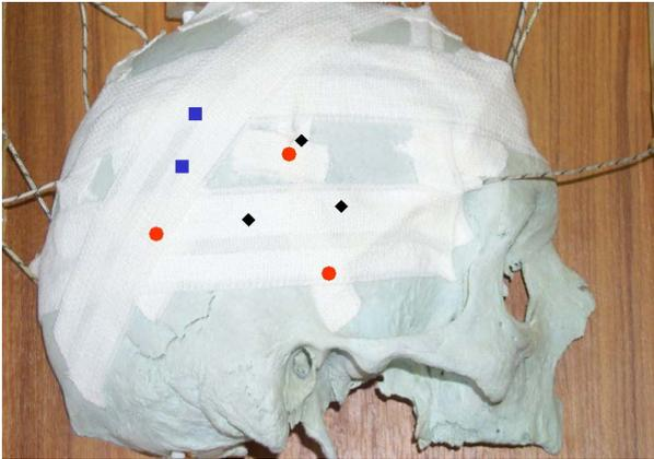
Figure 4. Location of the 8 thermocouples sensors. (on the outer surface ●, on the inner surface ◆, inside of the skull ■).
