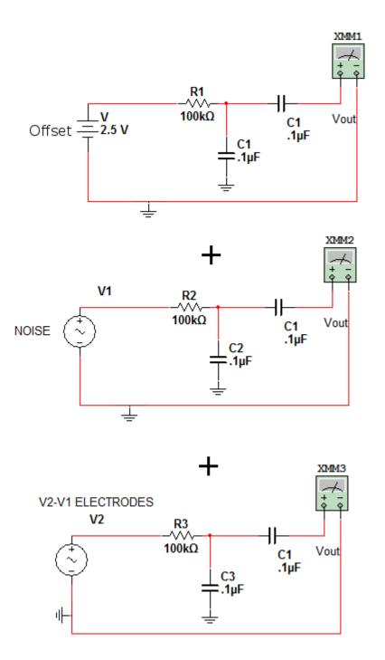
The output signal on the biomedical system should be a sum of the offset, noise, and the differential potential.
