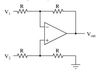
If all the resistor values are equal, this amplifier will have a differential voltage gain of 1. The analysis of this circuit is essentially the same as that of an inverting amplifier, except that the noninverting input (+) of the op-amp is at a voltage equal to a fraction of  $V_2$ , rather than being connected directly to ground. As would stand to reason,  $V_2$  functions as the noninverting input and  $V_1$  functions as the inverting input of the final amplifier circuit. Therefore:
