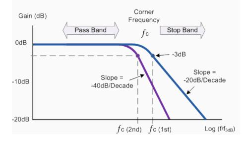
In practice, cascading passive filters together to produce larger-order filters is difficult to implement accurately as the dynamic impedance of each filter order affects its neighbouring network. However, to
