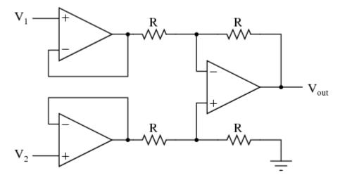
Now the  $V_1$  and  $V_2$  input lines are connected straight to the inputs of two voltage-follower op-amps, giving very high impedance. The two op-amps on the left now handle the driving of current through the resistors instead of letting the input voltage sources (whatever they may be) do it. The increased complexity to our circuit is minimal for a substantial benefit.
