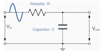
The reactance of a capacitor varies inversely with frequency, while the value of the resistor remains constant as the frequency changes. At low frequencies the capacitive reactance, (Xc) of the capacitor will be very large compared to the resistive value of the resistor, R and as a result the voltage across the capacitor, Vc will also be large while the voltage drop across the resistor, Vr will be much lower. At high frequencies the reverse is true with Vc being small and Vr being large.
