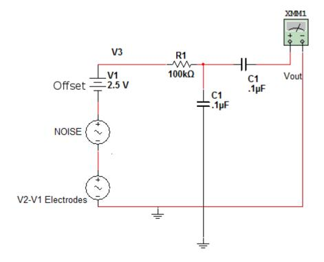
The system relies on three different factors: Offset, noise, and the differential voltage.
