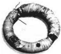
Figure 2.2 Michael Faraday and one of the coils he used in his studies on electromagnetic induction. Illustration of the first magnetic induction coil, sketched by Faraday in his laboratory notebook on 29 August, 1831, and an inset from the notebook.
