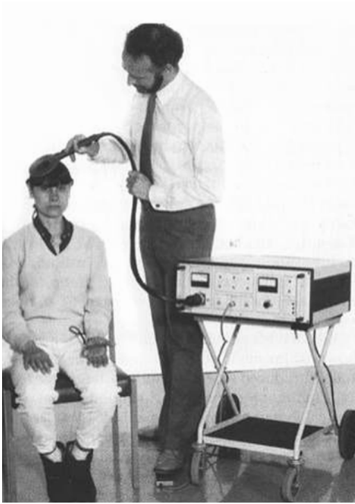
Figure 2.14 The world's first clinical magnetic stimulator in use at the University of Sheffield in 1985, England. (Reproduced from Barker, 1991.)
