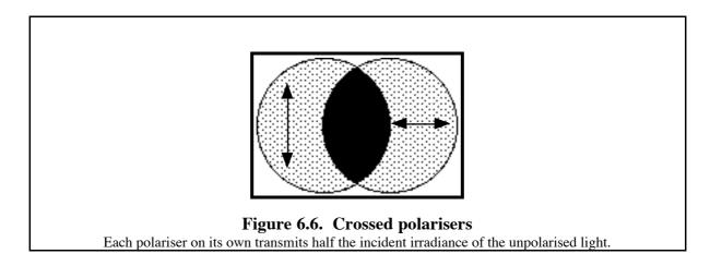
So far we have considered a polariser as something which produces polarised light. It can also be considered as a device for detecting polarised light. When it is used that way it may be called an **analyser**. For example, in the case of crossed polarising filters above, you can think of the first filter as the polariser, which makes the polarised light, and the second filter as the analyser which reveals the existence of the polarised light as it is rotated.
