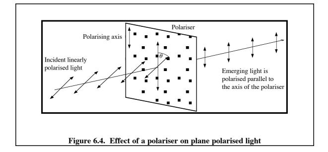
Many practical polarisers do not obey Malus's law exactly, firstly because they absorb some of the component with polarisation parallel to the polarising axis and secondly because some of the component polarised perpendicular to the axis is not completely absorbed.
