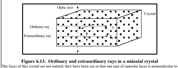
he faces of this crystal are not natural; they have been cut so that one pair of opposite faces is perpendicular t the optic axis while the other faces are parallel to the optic axis.
