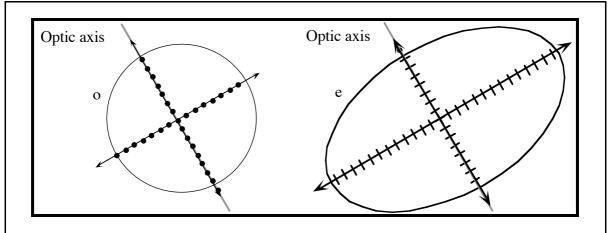
Figure 6.12. Polarisation of e and o waves
