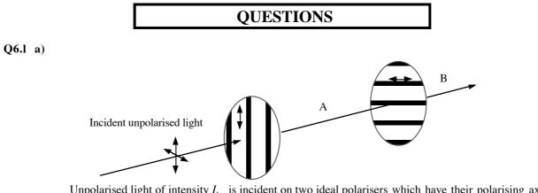
Unpolarised light of intensity  $I_{in}$  is incident on two ideal polarisers which have their polarising axes at 90° to each other. What are the polarisation and intensity of the light at A and B?
