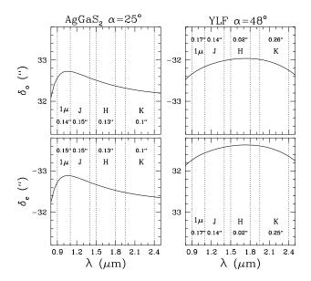
**Fig. 2.** Predicted separations (sky projected angles) between the "o" and "e" rays in AgGaS<sub>2</sub> and LiYF<sub>4</sub> (YLF) Wollaston prisms inserted at the  $\oslash$  22 mm pupil plane of NICS, the IR instrument for the Italian 3.5 m Galileo telescope. Note the large total separation of the beams,  $|\delta_{\rm o} - \delta_{\rm e}| > 1'$ , and the very small image elongation in the 0.9 – 1.1, J, H and K bands
