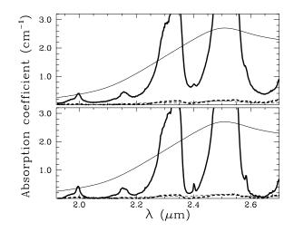
Fig. 4. Absorption coefficient of Calcite for the ordinary (solid lines) and extraordinary (dashed lines) rays at room temperature (upper panel) and 77 K (lower panel). The thin lines show the data available in optical handbooks (e.g. Bennet 1995) and which are based on the old measurements of Nysader (1909)
