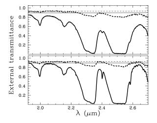
Fig. 3. Transmission of Calcite, thickness 9 mm, at room temperature (upper panel) and 77 K (lower panel), the solid and dashed lines refer to the ordinary and extraordinary ray, respectively, while the thin lines show the transmission expected including reflection (Fresnel) losses alone
