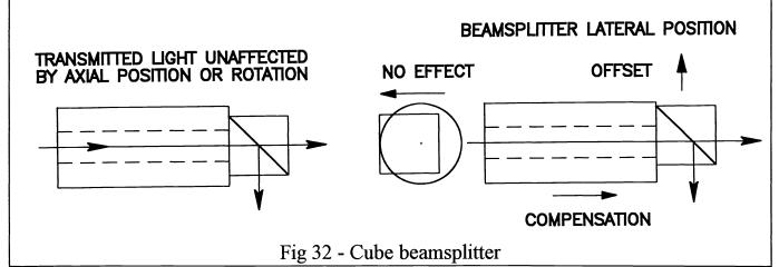
plane, an axial translation of the cylinder compensates. The cube location in the direction vertical to the plate is not critical. A beamsplitters may require a light trap, which can be built in a cylinder located in a fourth section of V. A mechanical method to locate cube beamsplitters is shown in Fig. 33.
