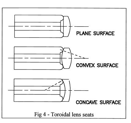
A single toroidal seat puts the center of curvature of one surface on axis, and two toroids completely center a lens, Fig. 5.
