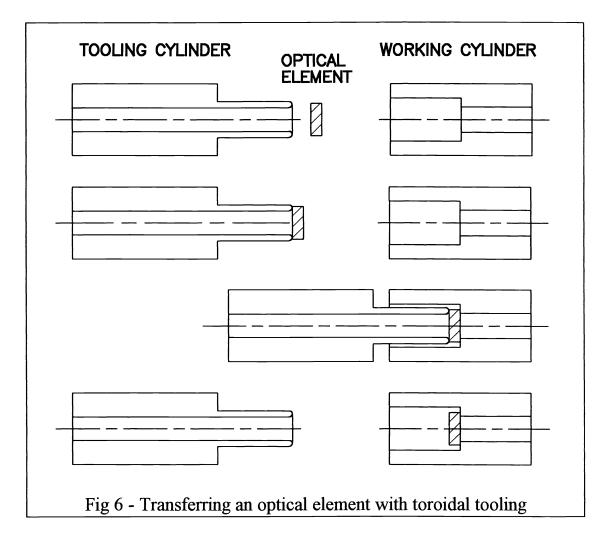
Only a small portion of a toroid is required for a given lens. Alternately, a toroidal surface can be devised to mount a family of lenses. To reduce contact stress, the profile of the toroid can be made close to that of the lens. Numerically controlled lathes can routinely produce such surfaces.
