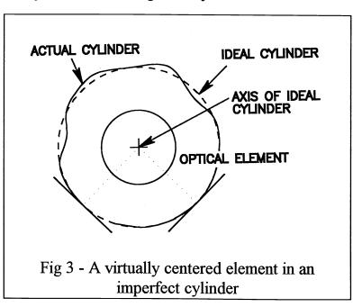
(In our shop we use an air spindle with 2 µinch runout. Tilt and centration are built in. The master cylinder, which was obtained from a gage house, is stainless steel 1" in diameter and 4" long, accurate to 1 µm. The master V has glass contact surfaces, 2" long. So centering to about a micron is done with ordinarily machined cylinders.)
