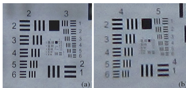
Figure 5. Lens resolution. (a) Initial state. (b) Focusing state.
