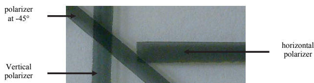
FIG. 10 Scene with 3 polarizers having different polarization orientation.
