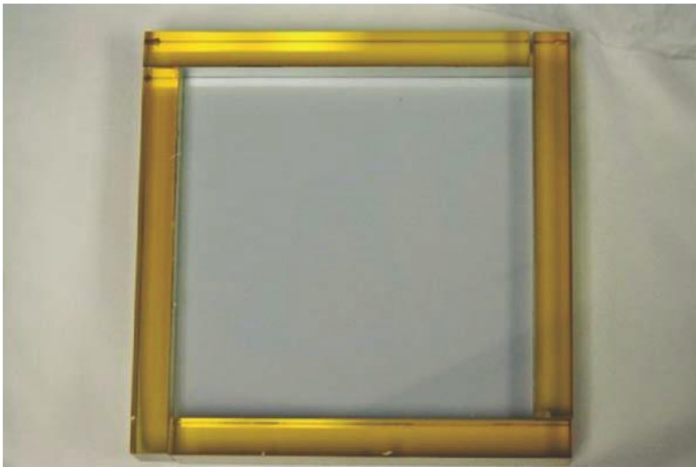
FIGURE 11.13 Ceramic Nd:YAG slab with cobalt-doped, epoxy-bonded edge cladding.
