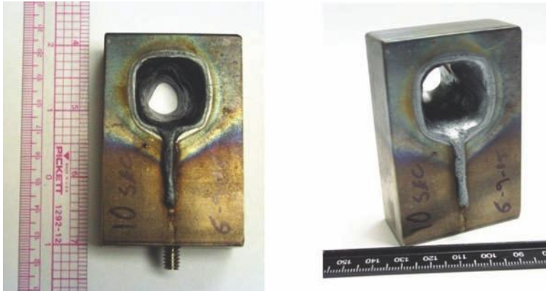
FIGURE 11.32 25 kW on a 1-in-thick carbon steel target for 10 s.
