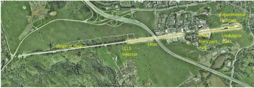
FIGURE 4.3 The Stanford Linear Accelerator Center with a layout of the Linac Coherent Light Source x-ray FEL. The LCLS utilized the final third of the SLAC linac with a new injector and undulator added. (Courtesy John Galayda)
