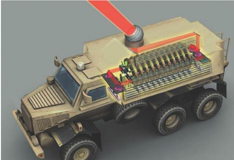
FIGURE 11.35 400-kW heat-capacity laser system on a mine-resistant, ambush-protected vehicle.
