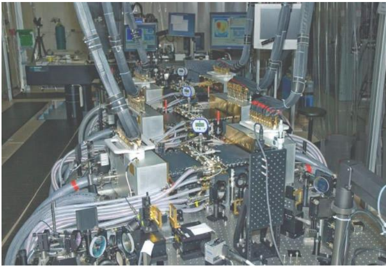
FIGURE 9.17 Three TZ-3 modules operating as a single-aperture power oscillator.
