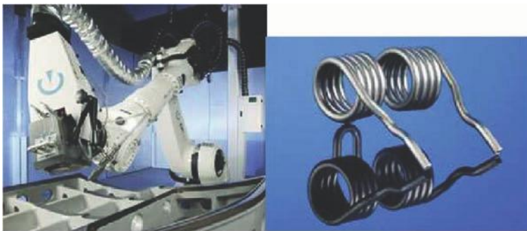
FIGURE 6.24 Laser hardening of tools and springs. (Courtesy of LaserLine)
