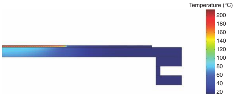
FIGURE 10.5 Calculated temperature for a Yb:YAG thin-disc; thickness 180 \mu\text{m} , mounted on a CuW heat sink with thickness 1 mm, pump spot radius 7.5 mm, and heat source per area 5.4 W/mm 2 , equivalent to 60 W/mm 2 absorbed power density.
