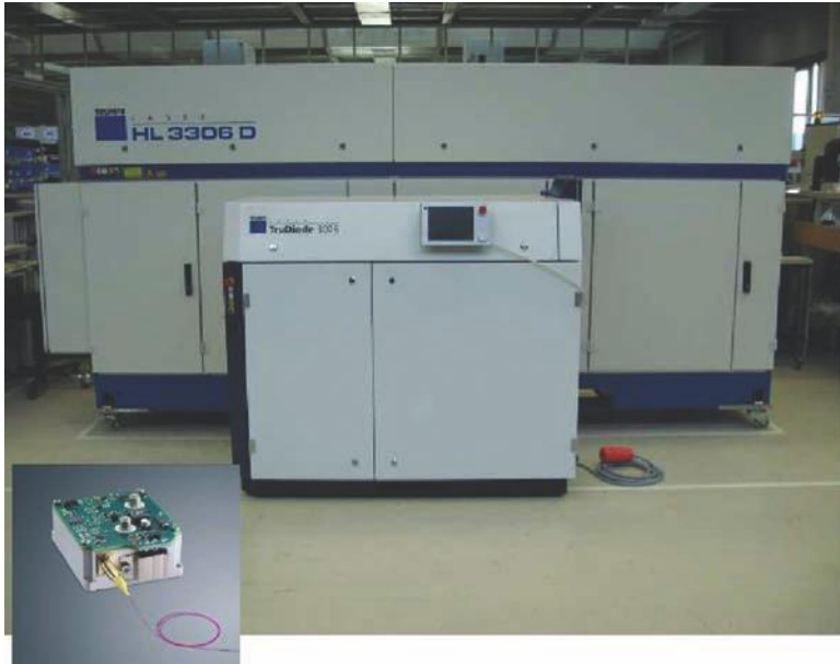
FIGURE 6.20 3-kW lamp-pump solid-state laser compared (back) with a 3-kW TruDiode system (front). The 100-W base module is shown in the inset.
