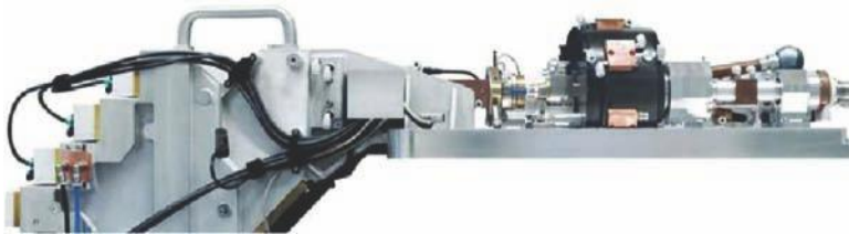
FIGURE 6.21 Multikilowatt diode-pumped disk laser: homogenized pump source (left) and laser cavity (right).
