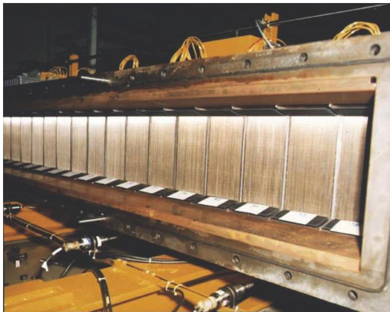
FIGURE 3.15 One of two MIRACL laser nozzle banks, consisting of 19 modules (not all shown).
