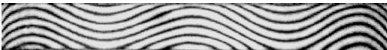
FIGURE 8.20 Typical 4-kW slab gain module OPD measured using a Mach-Zehnder interferometer operating at 658 nm. The zigzag axis is vertical, and the non-zigzag axis is horizontal.
