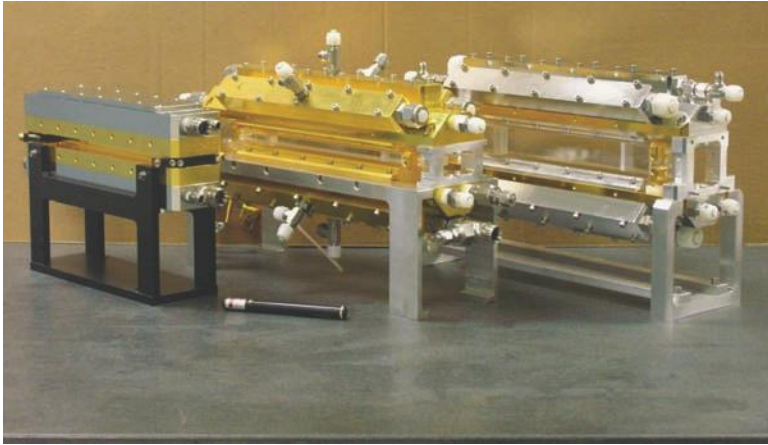
FIGURE 9.13 The three ThinZag modules: TZ-1, TZ-2, and TZ-3 (from left to right). Interestingly, there is not a significant size change in the modules as the power increases from about 1 kW laser output (TZ-1) to more than 15 kW laser output (TZ-3).
