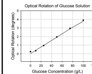
We used the gelatin PEM to measure the optical activity of a glucose solution, with concentrations varying between 0 and 100 g/L. The line is from the Hinds PEM and the black dots show the gelatin PEM results, indicating a close match between the two devices. A 637.5 nm laser was used for all measurements.
