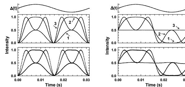
Curves 1, 2, and 3 of the left graphs are for quarter-wave, half wave, and three-quarter wave retardance amplitudes, respectively, when the offset retardance is zero. Curves 1 and 2 of the right graphs are for quarter-wave and half-wave retardance amplitudes when the offset retardance is a quarter-wave. Curve 3 of the right graphs is for input linear polarization that is aligned with the PEM's fast axis.
