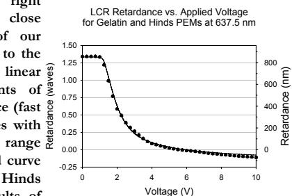
The graph on the right demonstrates the close similarity in results of our gelatin PEM compared to the Hinds PEM for linear retardance measurements of an LCR. LCR retardance (fast axis at horizontal) varies with voltage supplied over a range from 0 V to 10 V. Solid curve shows the results of the Hinds PEM. Dots show results of our gelatin PEM.
