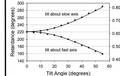
780nm half-wave plate tilted about the fast and slow axis. 637.5nm laser used. Solid curves show results of Hinds PEM. Dots show result of our gelatin PEM.
