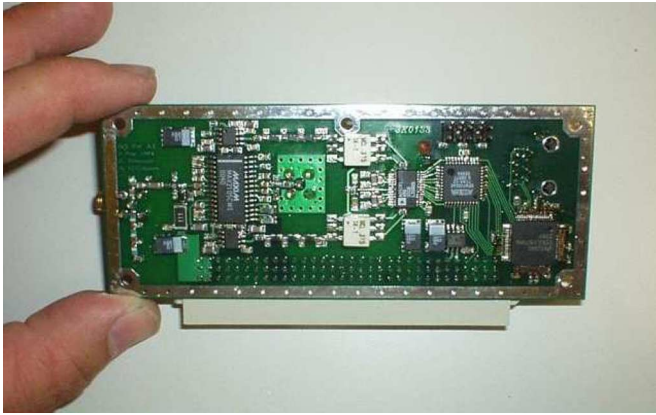
Fig. 7. DCR. Left to right: High-pass diplexer, Maxim MAX2105 direct conversion IC, Texas Instruments OPA643 IC output buffers, 7 MHz low-pass filters, baluns, Analog Devices AD9281 ADC, FPGA, LVDS transceiver IC. Jacks for RF, LO, and LVDS are on the opposite side of the board, which also forms one side of an enclosure. The enclosure is completed by an EMI shield, removed for this photo.
