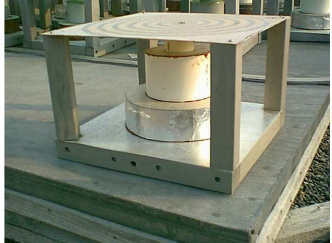
Fig. 3. Side view of a spiral antenna element.
