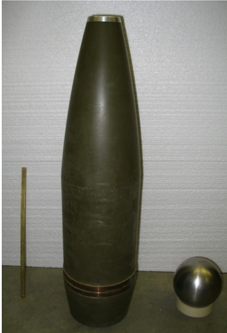
Figure 4.40: Three scatterers, modeled as perfect electrical conductors are shown. From left to right they are a rectangular pipe, a 155 mm artillery shell, and a calibration sphere.
