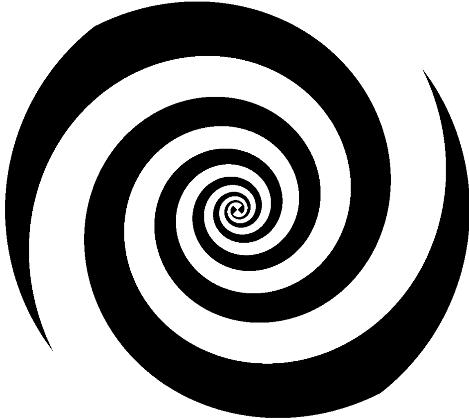
Figure 2.9: Numerical mesh used for verification of the FDTD model. This mesh has a uniform cell size of 0.2 mm and is 1184 \times 1184 \times 25 cells. Obtaining a suitable impulse response from the antenna required 6 ns of simulation time for the excitation used and required 2 hours of computer time on the 64 node cluster available at the time.
