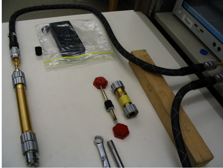
Figure 4.15: Measurement setup for the Baker-Jarvis dielectric measurements. A GR900 airline is used with a cut-out of the absorber placed on the center conductor. Because the calculation of \epsilon_r used only requires the S_{21} parameter, the exact distance to the beginning of the sample is not required. Only the length of the sample is needed.
