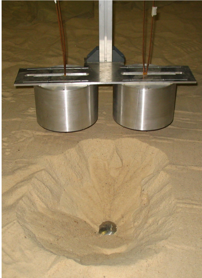
Figure 4.28: The bistatic pair is attached to a positioner facing toward the sand. A 6 cm radius metal sphere is placed in the ground. After burial, the sphere is 22 \pm 0.5 cm below the ground surface.
