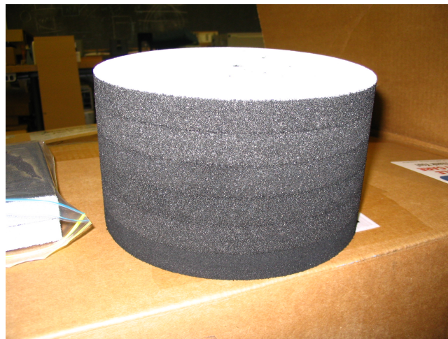
Figure 4.11: AN-79 absorber consists of six layers of carbon-loaded foam. Each layer from top to bottom has a higher carbon density to create a conductivity gradient for absorbing an incoming wave.
