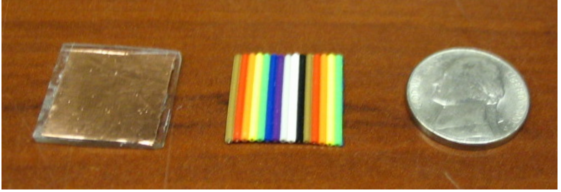
Figure 5.9: Scatterers chosen for illustrating the symmetry properties of the polarizability matrix. On the left, a square piece of copper tape is attached to Plexiglass. The scatterer is invariant under a 90^\circ rotation and should not conduct a significant amount of current along its thickness. In the center a square of ribbon-wire is used. The only significant direction of current flow is fixed by the direction of the wire. The nickel is included as a size comparison only. Each scatterer is a 2 cm by 2 cm square.
