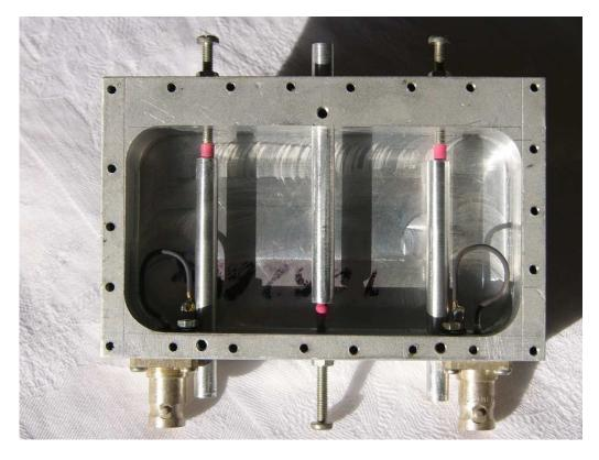
Figure 50. Interdigital filter for operation at 940 MHz, with top plate removed.
