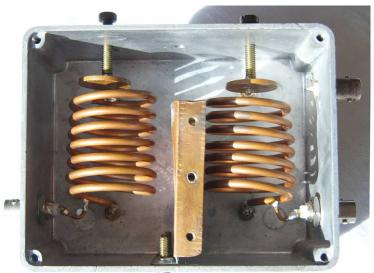
Figure 46. 101 MHz helical filter 1 MHz bandwidth
