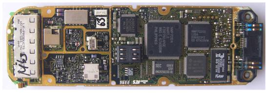
Figure 2. FR4 Multilayer Printed Circuit Board. (Nokia Mobile Phone).
