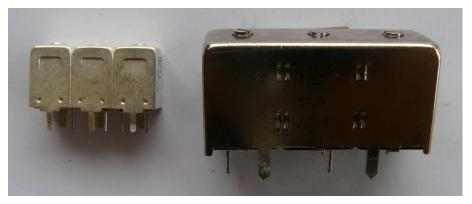
Figure 48. Commercial Helical Filters. Temwell Left, Toko Right.
