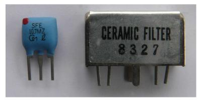
Figure 73. 10.7MHz ceramic IF filters.
