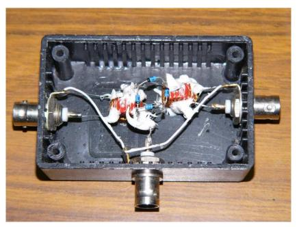
Figure 34. Construction of a Double Balanced Mixer for use in Practical Sessions.
