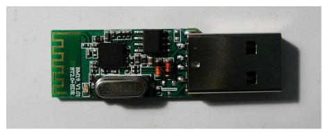
Figure 2. Typical Consumer RF Module. (Unbranded EDR Bluetooth USB Adapter)
