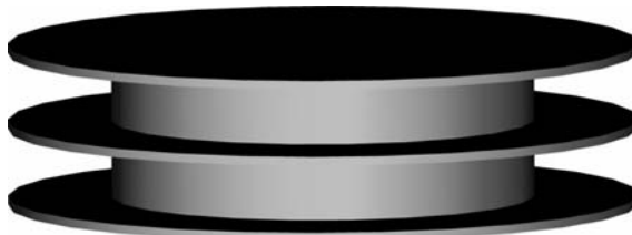
FIGURE 7-12 Ground plane with short-circuited radial transmission-line corrugations.
