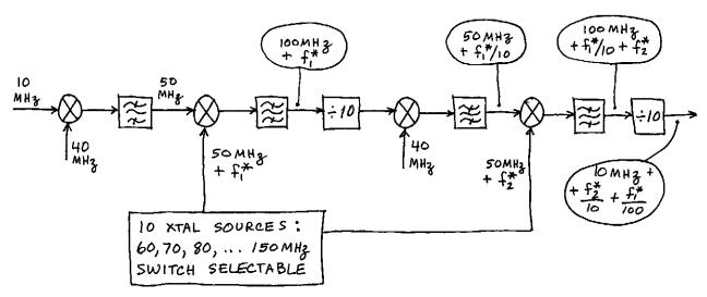
Two 10-position switches are used to select fit and  $f_2^*$  individually as 10, 20, 30, ... 100 MHz. a 10 MHz and a 40 MHz source are also needed.
