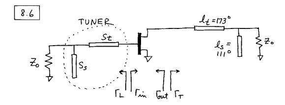
as in Example 8.4, choose  $\Gamma_L = 0.6 L - 130^{\circ}$ . Then Fout, Zout,  $\Xi_T$ ,  $L_t$ , and  $L_s$  are unchanged. Then we have the matching problem of using a stub-tuner to match 50 s.to  $\Gamma_L$ . The stub-susceptance is  $jbs = \frac{1}{2}1.56$ , for a stub-length of  $S_s = 0.158 \lambda$ . The line length is  $S_t = 0.004 \lambda$ .
