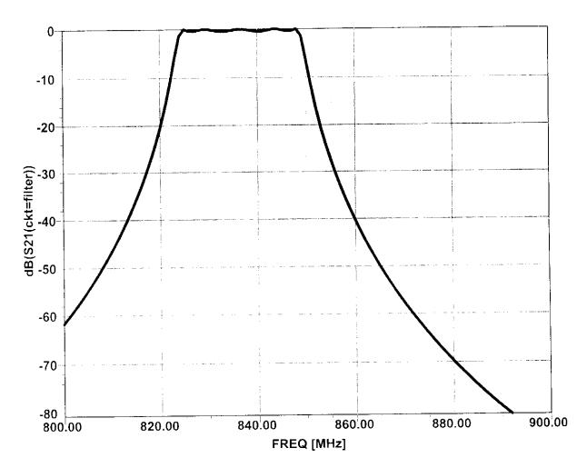
5.15 fo = 836.5 MHz, A=0.03, BANDPASS, 0.5dB EQUAL-RIPPLE, Zo=50x. CAPACITIVELY-COUPLED RESONATORS.
