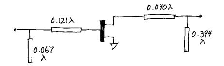
Serenade analysis gives  $G = 10.1 dB^{V}$  The return losses are  $RL_1 = -7 dB$ ,  $RL_2 = -6 dB$ . These mismatches serve to reduce the gain to 10 dB. The Smith chart plot of the relevant constant gain circles is shown below:
