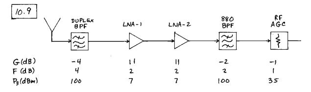
The attached FORTRAN code was used to compute the cascade values, and plotted below. The noise figure is about the same as for the original configuration, but P3 is lower by about 2.4 dB.
