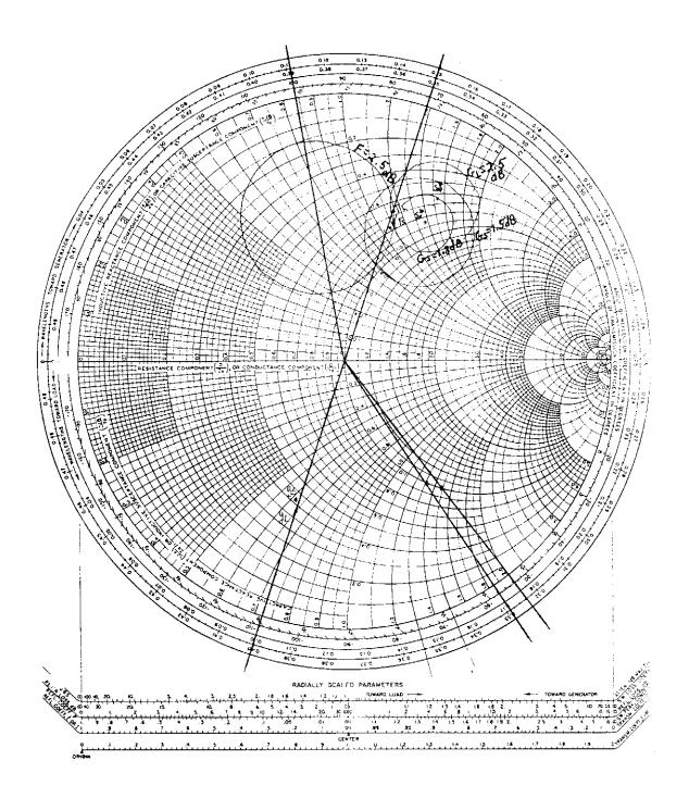
[6.17]  $S_{11} = 0.76 \underline{l169}^{\circ}$ ,  $S_{12} = 3.08 \underline{l69}^{\circ}$ ,  $S_{21} = 0.079 \underline{l53}^{\circ}$ ,  $S_{22} = 0.36 \underline{l-169}^{\circ}$  $\Gamma_{SP} = 0.797 \underline{l-187}^{\circ}$ ,  $\Gamma_{LP} = 0.491 \underline{l185}^{\circ}$ ,  $G_{P} = 10 dB$ . f = 1 G + 13.
