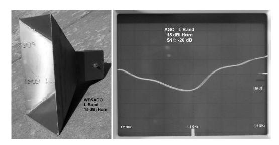
Appendances: Optimum 15 dBi pyramidal standard gain horn using smaller rectangular (2.6 x 5.6) waveguide, which cutoff is around 1.1 GHz (TE10). 6061 Al all wielded construction. This waveguide size (6 inches long) as shown above provided one of the better broad band return loss of the transitions tested. This illustrates that a variety of waveguide sizes from 5.6 to 8 inches wide can be tuned to work all measured better than -18 dB return loss.
