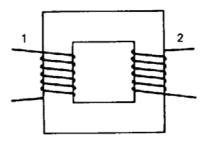
Fig.6.2. The arrangement of a simple transformer
