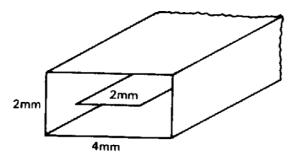
Fig. 7.9. A square coaxial transmission line
