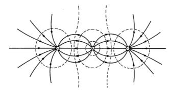
**Fig. 1.5** The field pattern around a positively charged wire flanked by a pair of negatively charged wires.
