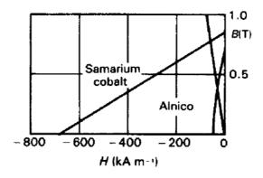
Fig. 5.18. The demagnetization curves for Alnico and samarium cobalt (SmCo<sub>5</sub>).
