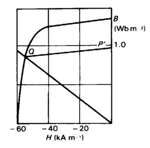
Fig. 5.12. The demagnetization curve for Columax.
