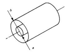
Fig. 1.7: The arrangement of an air-spaced coaxial line
