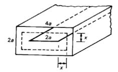
Fig. 6.6. A rectangular coaxial line with a strip centre conductor.
