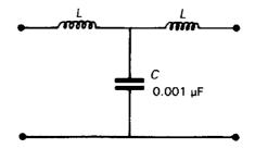
Fig. 7.6. One section of the pulse-forming network
