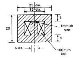
Fig. 6.3. A cross-sectional view of an inductor made with a cylindrical pot core of magnetic material.
