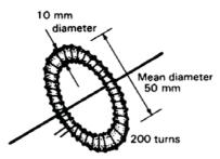
**Fig. 6.5.** A toroidal coil can be used as a transducer to measure the current in a conductor which passes through it.
