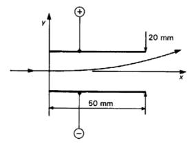
Fig. 1.13 The arrangement of a pair of electrostatic deflection plates for an electron beam.
