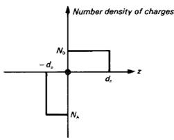
**Fig. 2.16.** The distribution of ionized donor and acceptor states in the depletion layer of an idealized p-n junction.
