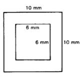
Fig. 2.14. Square coaxial electrodes
