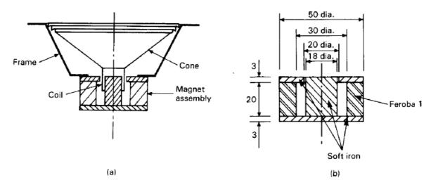
Figure 5.14(b) shows a cross-sectional view of a cylindrical loudspeaker magnet. Estimate the flux density in the air gap.
