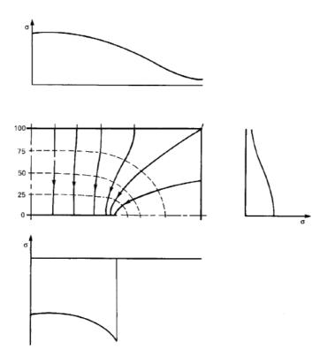
Fig. 2.12. The field map and charge density distributions derived from Fig. 1.18.
