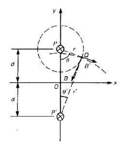
**Fig. 5.2** The calculation of the flux density at Q for the arrangement shown in Fig. 5.1 by replacing the iron sheet with an image conductor at *P*'.
