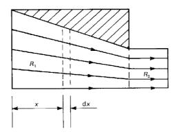
**Fig. 3.9** Approximate current flow lines to find an upper bound for the resistance of the strip shown in Fig. 3.7.
