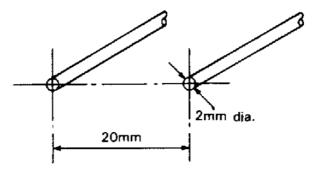
Fig. 7.8. Air-spaced two wire transmission line
