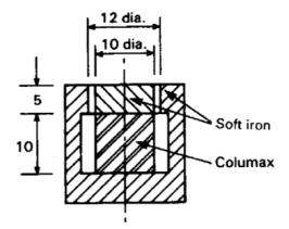
**Fig. 5.16.** The arrangement of a Columax loudspeaker magnet. Notice how the use of a magnet material with a higher energy product allows the permanent magnet to be put at the centre instead of outside as shown in Fig. 5.13(b).
