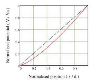
Fig. 1.14 The potential distribution in a space-charge limited diode
