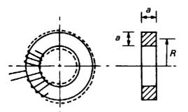
Fig. 6.4. The arrangement of a toroidal inductor.
