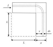
Fig. 3.5 Approximate current flow lines.
