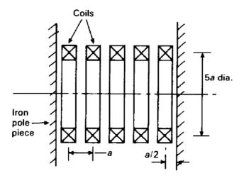
Fig. 5.3 The arrangement of a solenoid having a number of coils and iron pole pieces at either end.
