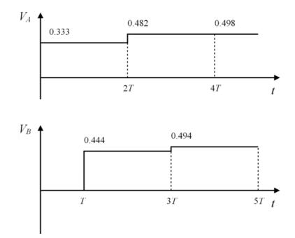
Fig. 7.5. Voltages across the line at A and B as a function of time for example 7.2
