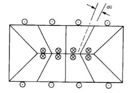
Fig. 6.7. An approximate current distribution in the rectangular coaxial line with a strip centre conductor.
