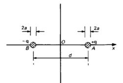
Fig. 2.3 Cross-sectional view of a parallel-wire transmission line
