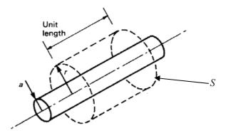
Fig. 1.8 A Gaussian surface for calculating the electric field strength around a line charge.
