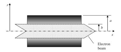
Fig. 1.12 The arrangement of an electron beam within a concentric conducting tunnel
