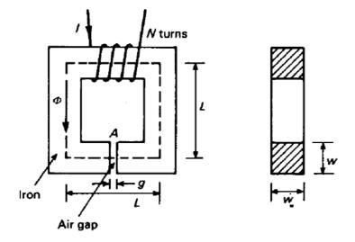
**Fig. 5.5.** A simple magnetic circuit made up of an iron core with an air gap in it. The magneto-motive force is supplied by a winding of *N* turns of wire
