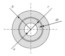
Fig. 3.1. Arrangement of a coaxial cable.
