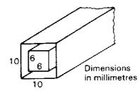
Fig.6.8. A square coaxial arrangement of electrodes
