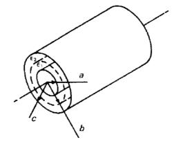
Fig. 2.7 A coaxial cable with two concentric layers of dielectric material between the conductors
