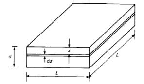
Fig. 3.2 Calculation of the sheet resistance of an integrated-circuit diffused resistor.
