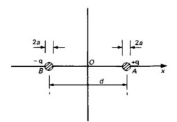
Fig. 1.9 A cross-sectional view of a parallel-wire transmission line.
