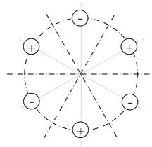
Fig. 1.4 Image charges for planes intersecting at 60°
