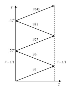
Fig. 7.4. Time of flight diagram for example 7.2
