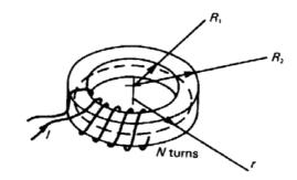
Fig 4.5. A coil wound on a ring-shaped former.
