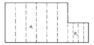
**Fig. 3.10** Approximate equiportential surfaces to find a lower bound for the resistance of the strip shown in Fig. 3.7.
