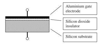
Fig. 2.1 Arrangement of layers in a MOS transistor.
