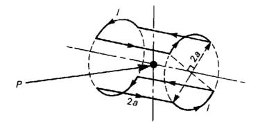
Fig. 4.4. The arrangement of a pair of saddle coils.
