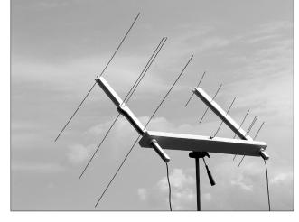
Photo 4: Crossboom and tripod with uplink and downlink antennas ready for action.
