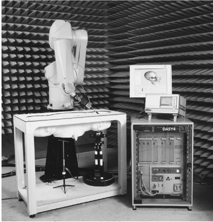
FIGURE 11.10 DASY4 dosimetric assessment system. (From SPEAG, Switzerland.)
