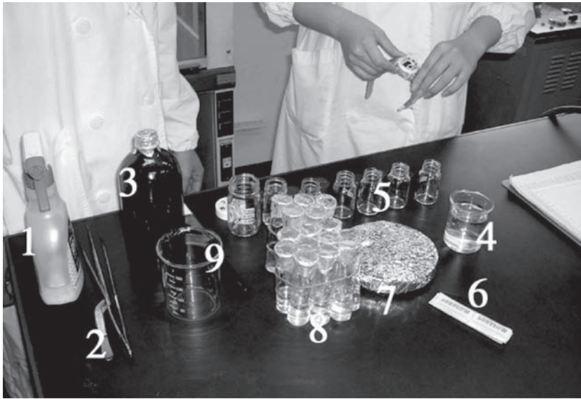
Fig. 1. The materials needed for sterile culture. (1) 70% EtOH, (2) forceps, (3) autoclaved sterile distilled water, (4) sodium hypochlorite solution, (5) 30-mL glass vial, (6) Parafilm, (7) 120-mm glass dish containing filter papers, (8) medium, and (9) beaker for waste fluid.
