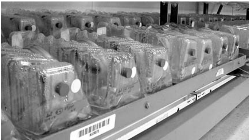
Figure 2: Rectangular vessels facilitated a slow moving wave of media to migrate the length of the vessel with the motion of the shelf.
