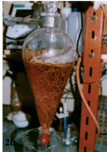
Figure 2: Results from (2a) simple airlift bioreactor of conical shape made of separation funnel (2b)
