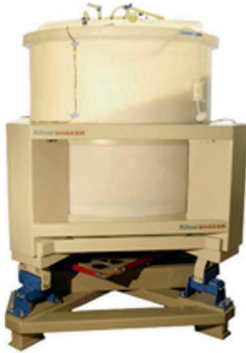
Fig. 12 A 2,000-L disposable shaken bioreactor system with a working volume up to 1,000 L. Shaking diameter: 10 cm, shaking speed: 40–45 rpm
