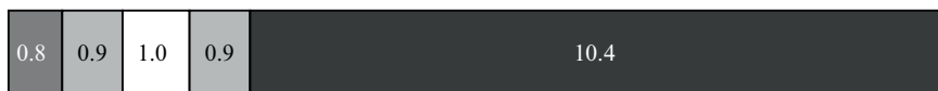
Fig. 7 Cross section through the different bag layers, Polyester ( dark grey filled square ), Tie ( light grey filled squares ), EVOH ( open square ), PE ( filled square )
