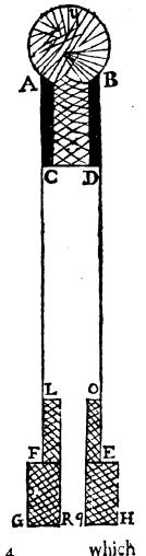
which bottom will be a Guide to the Piercer to be just in the middle of the Rocket, make a mark in your Piercer to be a guide to bore always an equal depth, then take your Rocket out of the Mould, open the hole with a Taper bit, and your Work is done, thus you may do for all fizes of Rockets.
