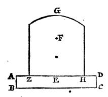
You may cut the Charger ABCDH GZA in Paper, then it may be made in Copper, Close A to D, and B to C, Sodder both ends together; bring HGZ into more than half a round, and AB and CD in a round, put it then upon a Handle, then it is fit for use.
