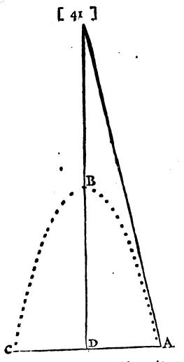
In the Parabola ABC, Let AC be equal to 330 Yards, AD equal to 165 the Angle DAE 78 degrees, then in the right Angled Triangle EDA.
