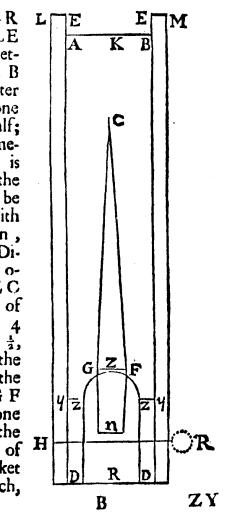
ZY one fixth of the Diameter of the Rocket a quarter of an Inch, the thicknels of the Case, DYZGCFZYD the bottom of the Rocket-Mould with the Needle to be put in and taken out; RH a Pin of Iton to fix the Mould and Bottom together.
