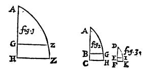
In the Parabola AHZ let AG be 2608, and AH3377; then GZ and HZ are the Velocities of the equal and unequal Ranges. Toricellius 22. Prop. de motu projec. lib secund.
