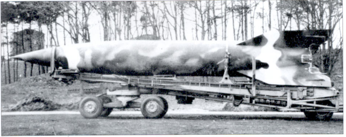
An A-4B is seen here on a Meillerwagen in the experimental June 1943 camouflage scheme. Most of this production run was expended in tests from Peenemünde and Blizna in 1943. (MHI)
