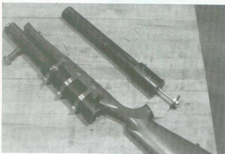
Two models of home-built 40mm weapons: M79 (left) and M203 (right) ready to be attached to a rifle.
