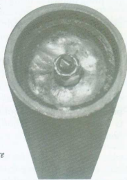
Completed firing pin assembly installed in breech pipe. Note screwdriver slot and secure braze holding assembly to pipe.
