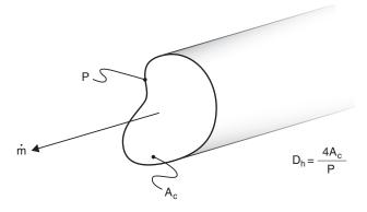
**Figure 7.9** Flow in a noncircular duct.
