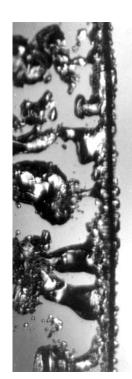
3.45 cm length of 0.0322 cm diam. wire in methanol at 10 earth-normal gravities. methanol at 10 earth-normal gravities.  $q=1.04\times10^6 \text{ W/m}^2$
