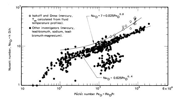
**Figure 7.8** Comparison of measured and predicted Nusselt numbers for liquid metals heated in long tubes with uniform wall heat flux,  $q_w$ . (See NACA TN 336, 1955, for details and data source references.)
