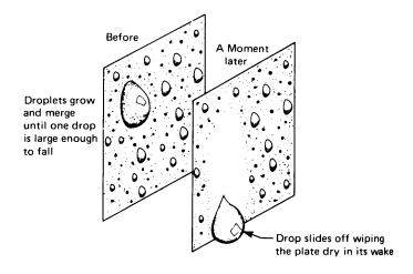
$\boldsymbol{a.}$  The process of liquid removal during dropwise condensation.
