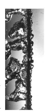
3.75 cm length of 0.164 cm diam. wire in benzene at earth-normal gravity.  $q=0.35\times10^6~\mathrm{W/m^2}$
