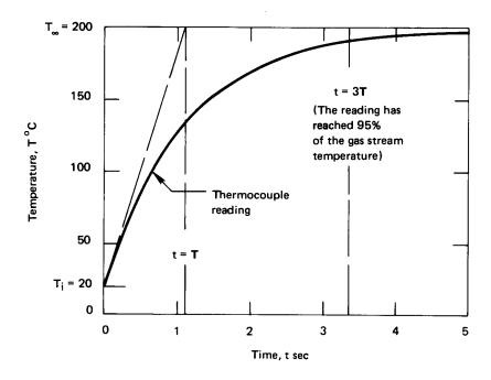
**Figure 1.12** Thermocouple response to a hot gas flow.
