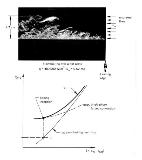
Figure 9.17 Forced convection boiling on an external surface.
