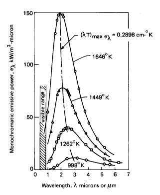
**Figure 1.15** Monochromatic emissive power of a black body at several temperatures—predicted and observed.
