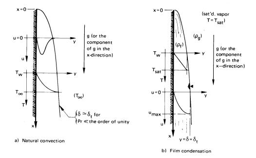
**Figure 8.1** The convective boundary layers for natural convection and film condensation. In both sketches, but particularly in that for film condensation, the y-coordinate has been stretched.
