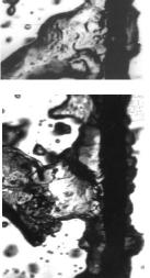
$\boldsymbol{b}.$  Two views of transitional boiling in acetone on a  $0.32\ \mathrm{cm}$ diam. tube.
