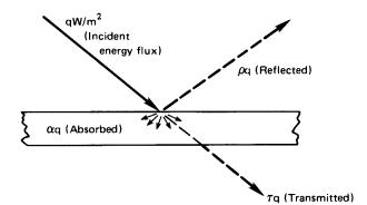
**Figure 1.14** The distribution of energy incident on a translucent slab.
