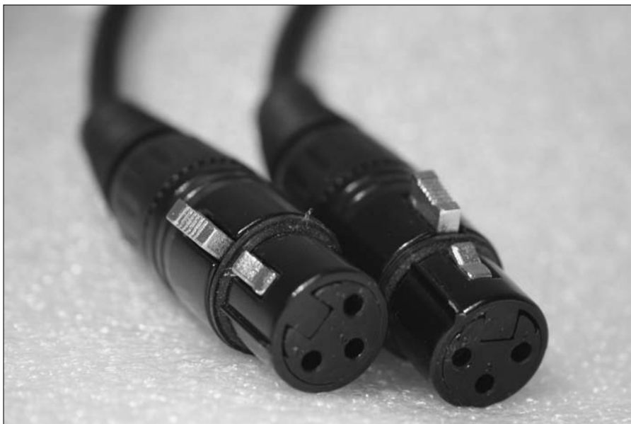
Figure 11-1: Two XLR connectors, one for the left, the other for the right.
