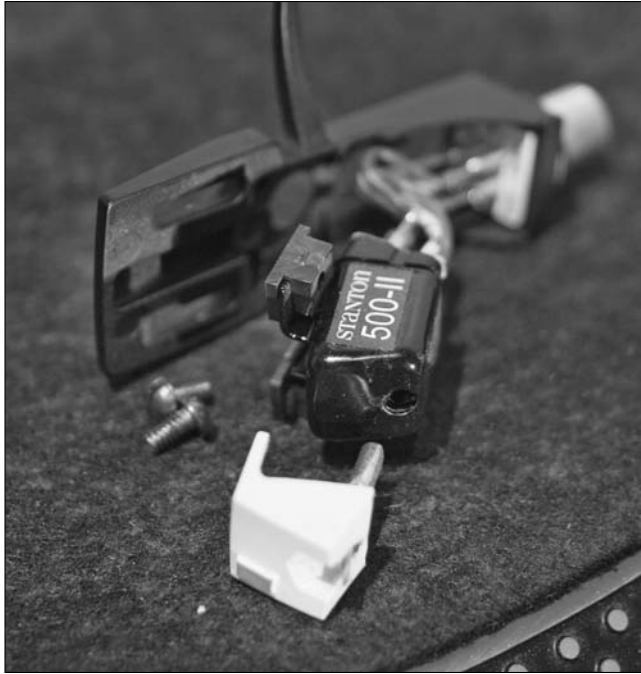
Figure 6-3: A disassembled needle and cartridge with a Technics headshell.
