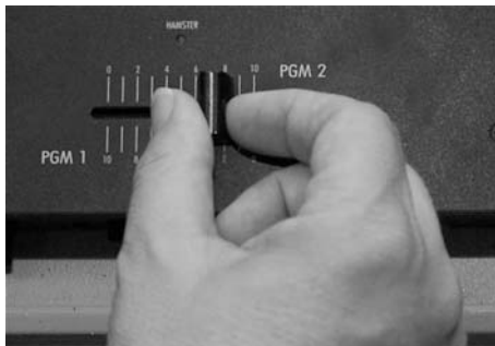
Fig. 19.50. Flick the fader momentarily open with the index finger.
