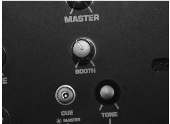
Fig. 15.20. The volume pot for the DJ booth's monitor system.
