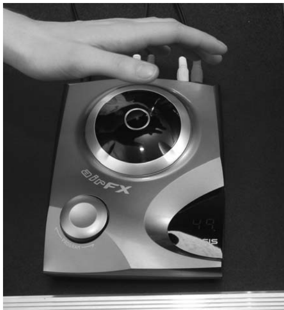
Fig. 11.11. The Alesis Air FX sends a beam of infrared light out of the top, then uses sensors in the dome which see the light reflected off of your hand.
