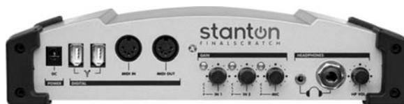
Fig. 9.3. Stanton's ScratchAmp 2 supports digital recording as well as play back.
