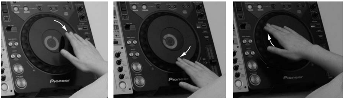
Fig. 15.58, Fig. 15.59, and Fig. 15.60. Spin the platter/jog wheel clockwise with your finger. Be sure you're in CD (not vinyl or scratch) mode. This will speed up playback momentarily.
