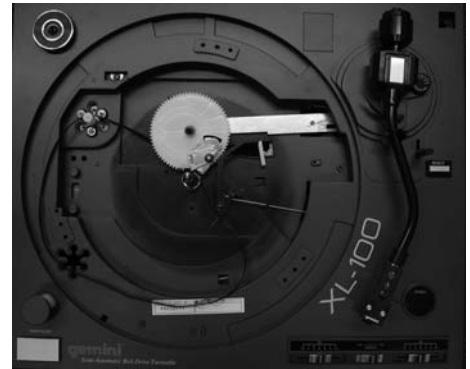
Fig. 7.7. An inexpensive belt-driven mechanism.
