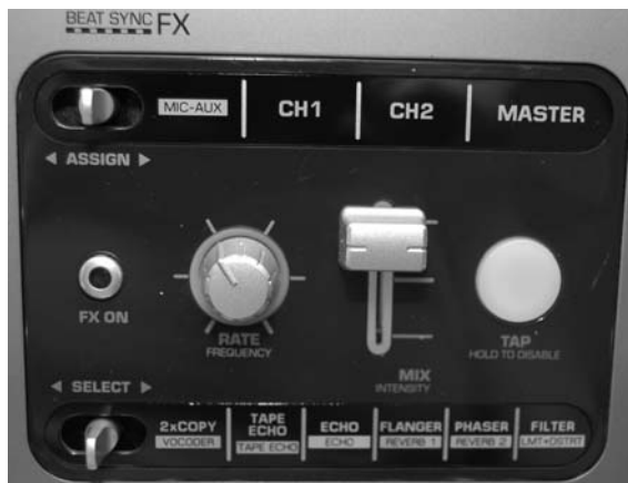
Fig. 11.10. The effects section of the Numark DXM06 digital mixer. Digital mixers often incorporate onboard effects into their design.
