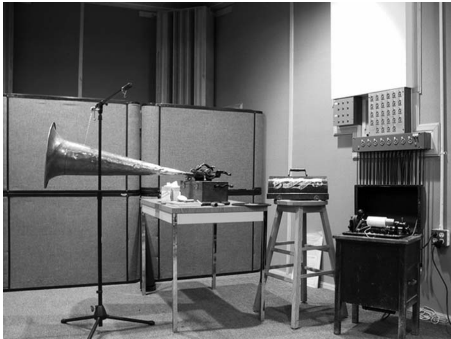
Fig. 1.1. The Edison wax cylinder recorder. This device collected sound through a horn, then translated sound pressure levels into movements of a diaphragm, which vibrated the connected stylus, cutting tiny grooves in a rotating wax cylinder.
