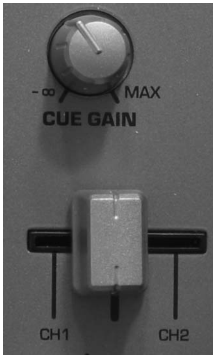
Fig. 15.18. Some two-channel mixers, like this Numark DMX 06, include a mini crossfader, which lets you select and blend between sources in the headphones independently of the master crossfader.
