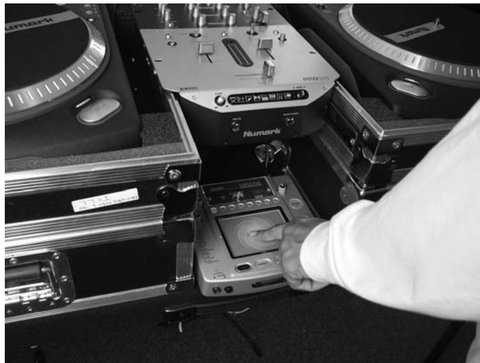
Fig. 14.3. Suspending the mixer has the added benefit of giving you space underneath for an effects unit such as the Korg Kaoss Pad.
