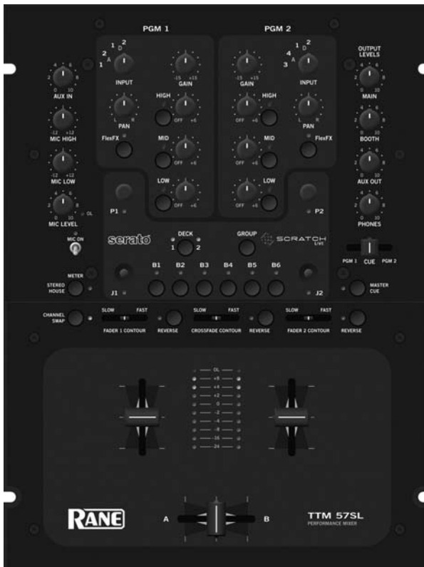
Fig. 11.13. The Rane TTM 57SL can convert the input from Serato Scratch Live time code control records into digital signals to control the SSL software without the need for additional hardware.
