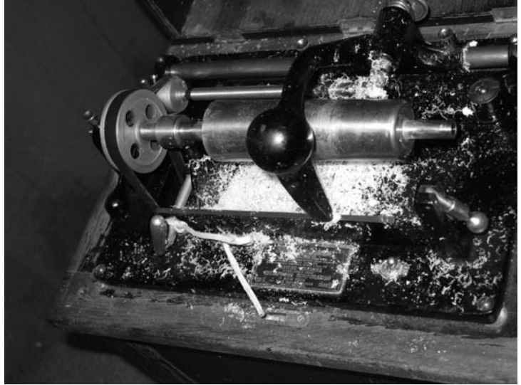
Fig. 1.2. Disc-shaving machine. The shaving machine would smooth out the shallow grooves of the previous recording, making the wax cylinder smooth again and ready for new material.
