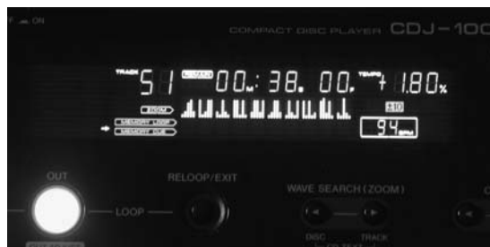
Figs. 8.4. & 8.5. The visual location interfaces of the CDJ-1000; the platter and the waveform display.
