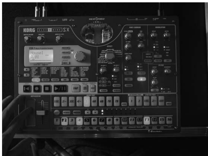
Fig. 10.5. The ESX-1 Electribe features vacuum tubes on the output stage, a ribbon, and slider control.
