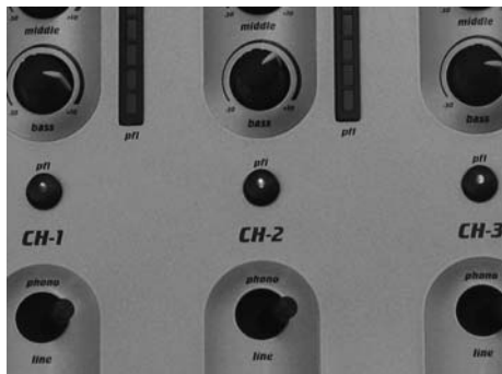
Fig. 15.16. "PFL" stands for "Pre Fader Level." This button lets you send a channel's pre-amplified signal to the cue section (thus hearing it in the headphones) even if the channel fader is all the way down.
