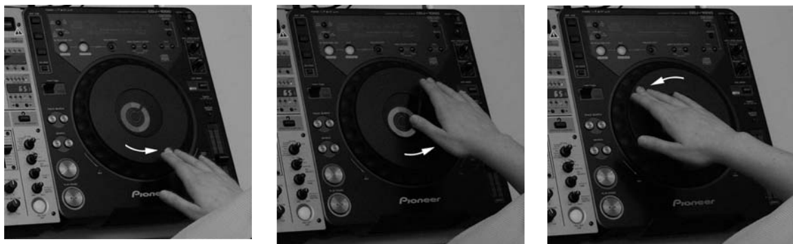
Fig. 15.64, Fig. 15.65, and Fig. 15.66. Spin the platter/jog wheel counter-clockwise with your finger. Be sure you're in CD (not vinyl or scratch) mode. This will slow down playback momentarily.
