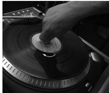
Fig. 15.42, Fig. 15.43, and Fig. 15.44. Give the spindle a few spins between your thumb and index finger, slightly faster than the platter is spinning on its own.
