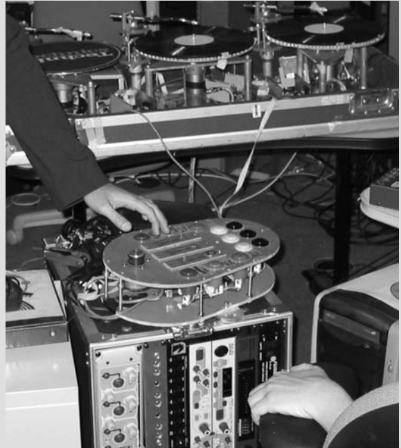
Fig. 13.3. The dedicated interface for the current DJ-I-Robot includes three crossfaders, and a knob to control the movements of any or all of the platters.
