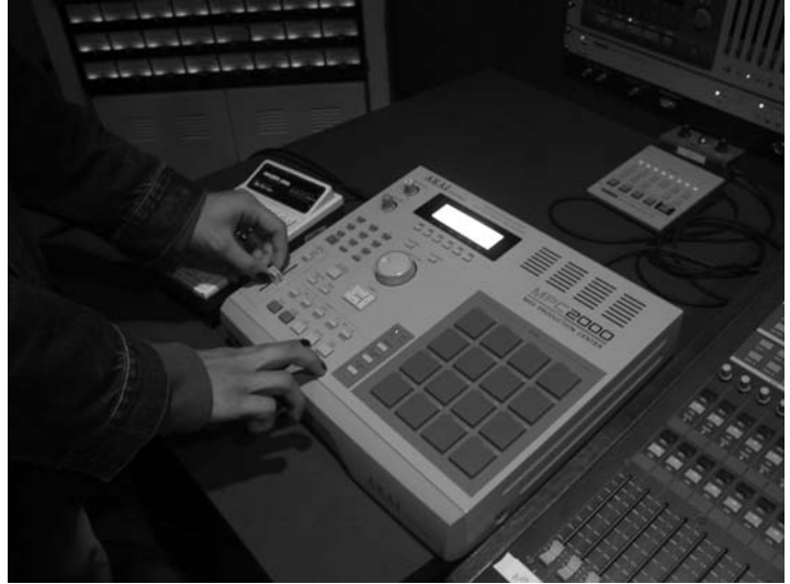
Fig. 10.3. The popular Akai MPC2000XL can read sample CDs of many formats through its SCSI port.
