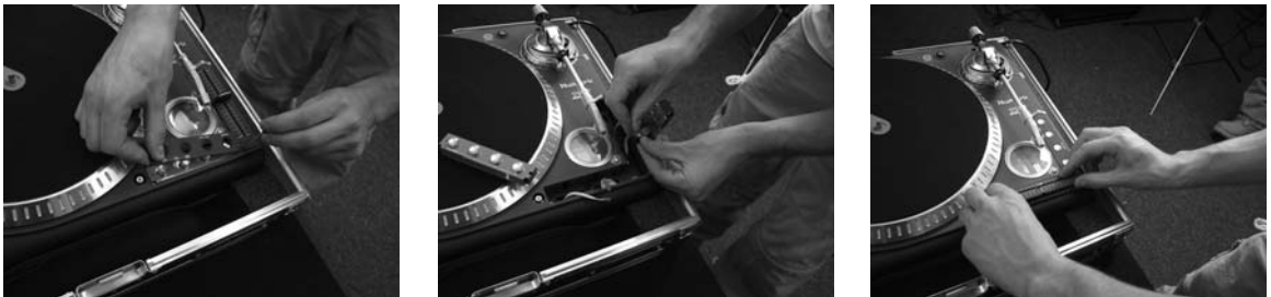
Fig. 7.11, Fig. 7.12 and Fig. 7.13. Switching the position of the pitch fader and the buttons on the TTX.
