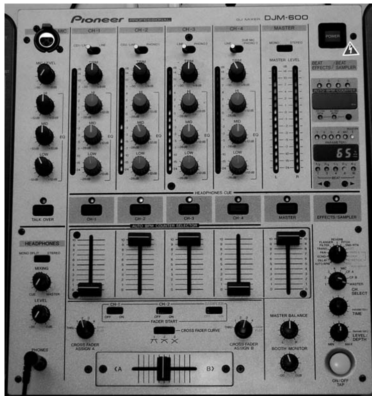
Fig. 11.7. The Pioneer DJM-600 includes an extensive array of features, including an onboard effects section, and a digital sampler.
