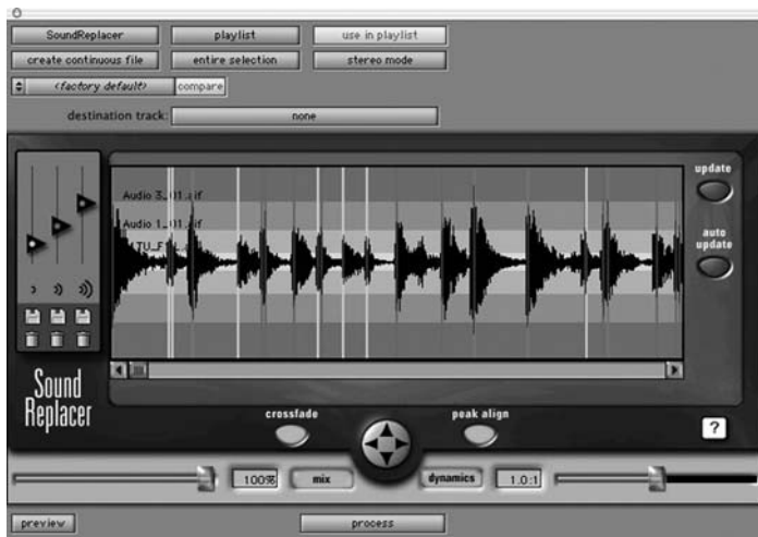
Fig. 9.13. Sound Replacer lets you keep a performance while replacing less-than-stellar sounds with new samples.
