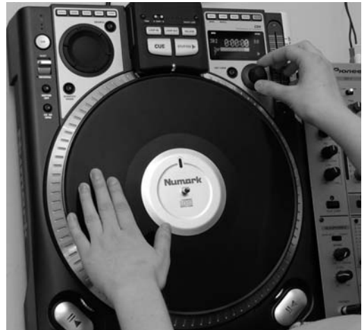
Fig. 15.30. Setting the beginning of a track to 12 o'clock on the metal label's marker on the CDX.
