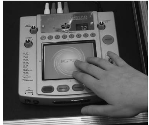
Fig. 11.12. The Korg Kaoss Pad senses the touch of your fingers on an X/Y-axis, and adjusts effect parameters accordingly.
