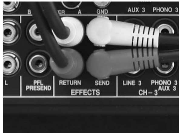
Fig. 11.9. An effects loop consists of a send and a return.
