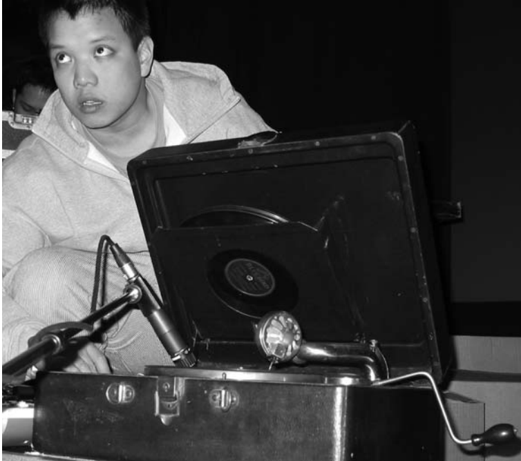
Fig. 1.3. Kid Koala with his vintage Victrola. Notice the massive tone arm, the manual crank, and the storage space for records in the lid.
