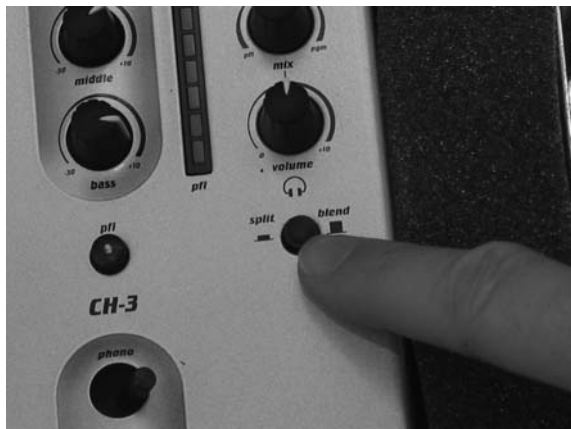
Fig. 15.21. The split button can help you keep track of what's happening on which record.
