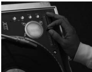
Fig. 15.45, Fig. 15.46, and Fig. 15.47. Momentarily slow down the record using the pitch adjustment control.
