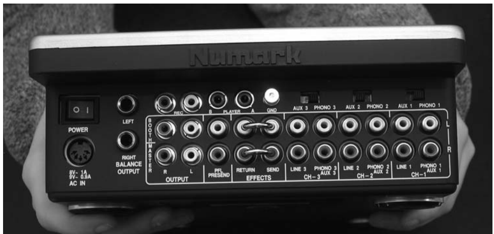
Fig. 11.8. The back panel inputs and outputs on the Numark Matrix 3 mixer.
