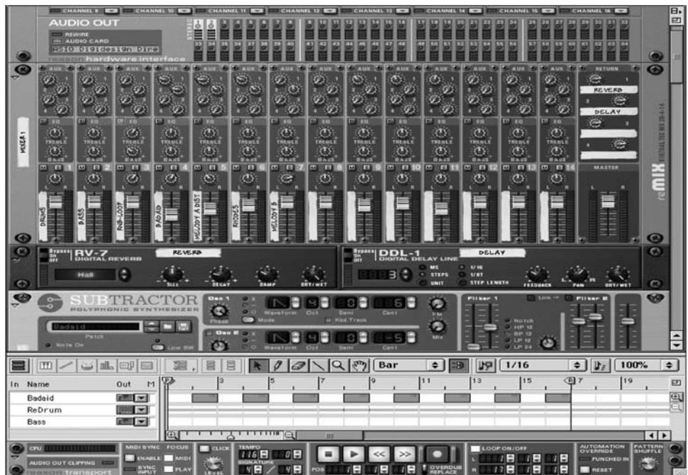
Fig. 9.9. Reason's interface resembles a rack of audio and MIDI hardware. You can even look behind the rack to check (and change) connections with virtual patch cables.
