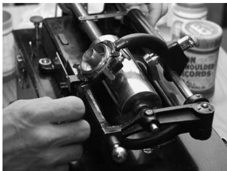
Fig. 7.2. With the horn removed, the diaphragm of the wax cylinder machine becomes visible.
