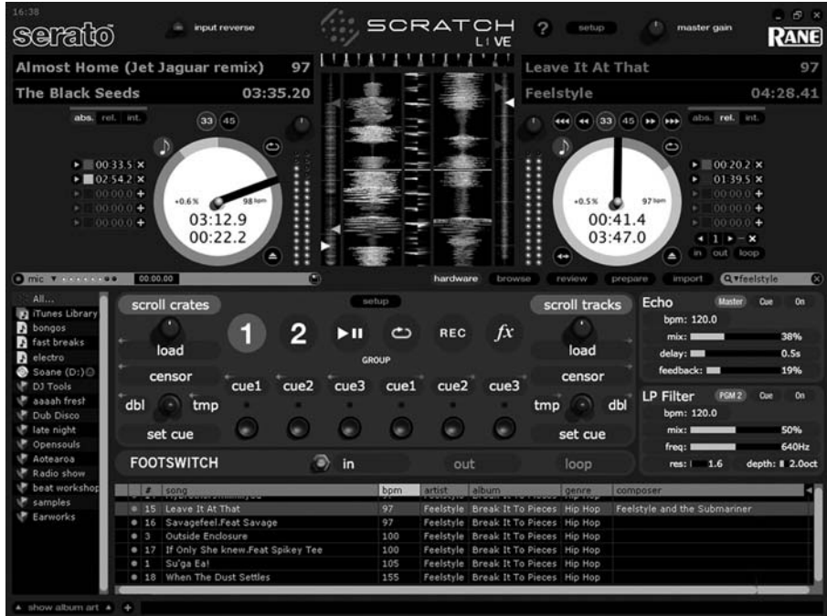
Fig. 9.4. Serato Scratch Live gives the user four different views of the music's waveform, the Tempo Matching display across the top, the Track Overview display along the sides, the Main Waveform display (the largest waveforms giving current position), and the Beat Matching display in the center.
