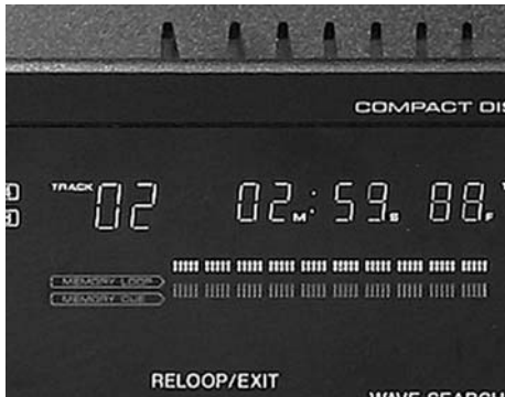
Fig. 15.7. A digital read-out of the track number, and the elapsed or remaining time of the track.
