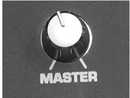
Fig. 11.3. The pot, a rotary control which adjusts audio signals by spinning clockwise or counter-clockwise.
