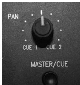
Fig. 15.17. This "cue" rotary pot controls the proportion of channel 1 versus channel 2 signal sent to the headphones.
