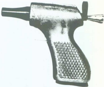
The C.I.A. 9mm Zip Gun is similar to the .45 Liberator in concept and design. The screw barrel leading has aluminum grips with space for extra cartridges. This photo has a 'horse collar' safety applied.
