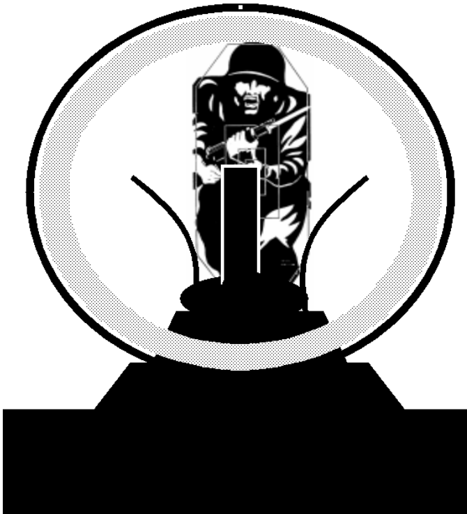
Figure 3-17: Correct Sight Picture—Iron Sights
