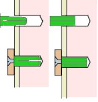
Lightweight blocks can be drilled very easily using a hand-brace or a power drill without hammer action. A risk with these blocks is that they are not very 'forgiving', a small amount of pressure in the wrong direction and the drill bit will be away where you never intended it to go.
