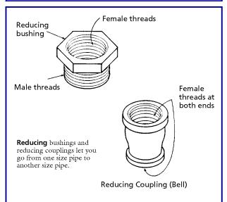
Fittings include tees, elbows, couplings, and unions. The fittings come in one size, as well as in a reducing size. That is, while the fitting will have one size to accommodate the pipe you are using, there will be one or more connections that are smaller. An example would be a 1/2-inch tee fitting that has a "straight through" size of 3/4-inch, while the connection at right angles would be 1/2- or 3/8-inch for the connection that supplies water to a sink or basin.
