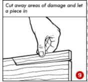
Wood fillers can be used to fill fairly deep holes by building up layers successively after the previous one has dried. However, they should not be used for large areas. These need additional wood 'let in' to the damaged area, after the rotted or damaged area has been cut away, leaving only good wood (9). Total
