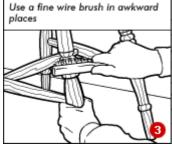
It may be necessary to use several applications of stripper to get into small crevices, and this is often best achieved by rubbing the area with paint stripper on wire wool by hand. A small wire brush (like those used for suede shoes) or a toothbrush can also be useful
