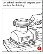
Orbital sanders come in various sizes and are used for finishing larger areas (6). Some are also designed to reach into very small spaces. These are called detail sanders.
