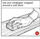
After you have stripped the timber, it must be prepared for finishing by sanding, either by hand or with an orbital sander. When hand sanding, it's useful to wrap the sandpaper around a cork block. This helps to create a flat surface and protects the user's fingers (5).
