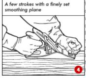
Wood that has been discoloured by age, weathering or fingermarks can often be brought back to life by taking off a few light shavings with a finely set smoothing plane. You must always work with the grain of the wood to avoid tearing out (4)
