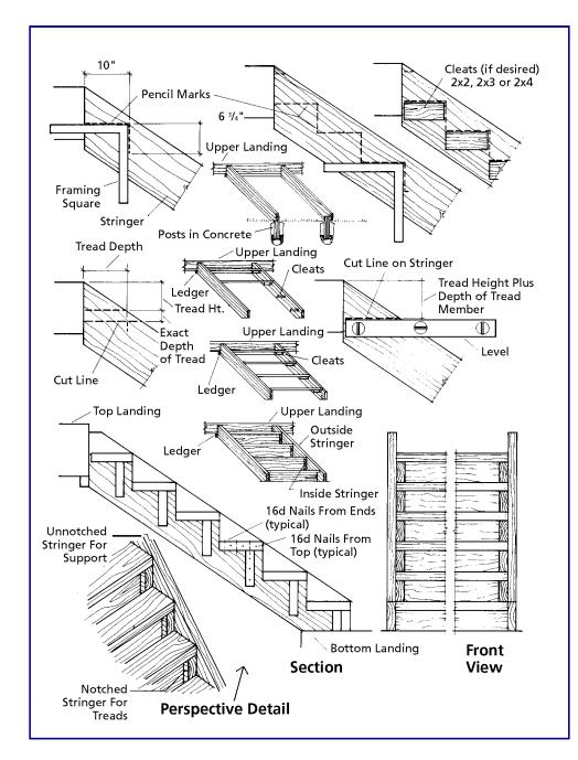
**Ground Exit.** If the last step down exits to the ground rather than to another deck surface, nail on the lowest cleats 2 inches from the top edge of the stringers, flush with the cut on the end of the stringers, and square from this cut.
