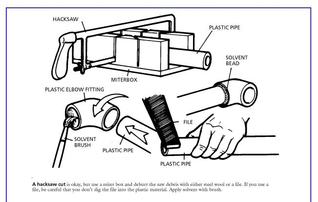
The pipe should be cut as square as possible, but squareness is not as critical as for rigid pipe. However, get it as square as you can. It is recommended that you cut this pipe with a hacksaw in a miter box and deburr it with sandpaper.
