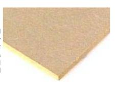
blockboard, MDF contains no internal voids, and will produce better edges providing that it is correctly machined.
