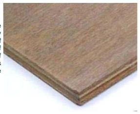
more veneers used, the stronger the plywood. Both the type of glue and veneers determine the suitability of a sheet for a particular application. The finish quality of plywood varies enormously, some have attractive grains while others can have a large number of knots.
