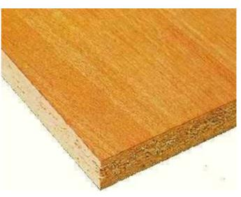
sheets so that the four decorated edges do not need to be cut. Thicknesses range from 12 to 25 mm.
