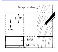
Story pole is a board marked with desired thickness of mortar joints and actual thickness of bricks to check the courses.
