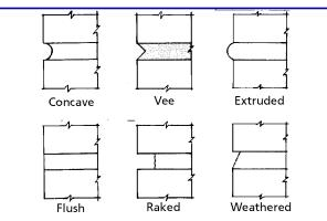
Mortar joints can be finished in many different ways, as illustrated. A round jointing tool forms the most popular finished joint—concave. Metal jointers are used to finish most joints; flush joints (flush with brick surface) are troweled. Avoid raked joints in areas of severe weather.
